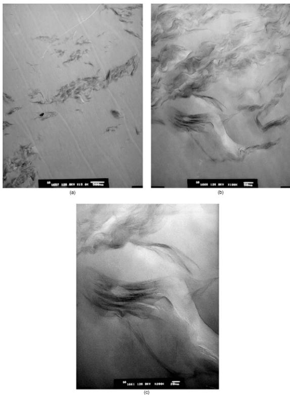
Fig. 3. (a) TEM image of SbC16 PS nanocomposite at low magnification. (b) TEM image of SbC16 PS nanocomposite at higher magnification. (c) TEM image of SbC16 PS nanocomposite at highest magnification.
