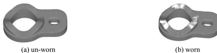
**Figure 3:** Representative surface profile of an (a) un-worn and (b) worn hinge cam.
