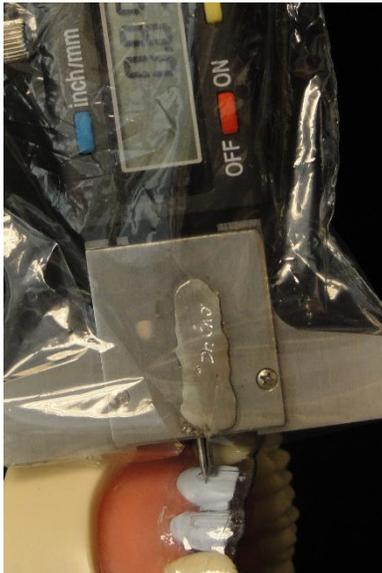
Fig. 6. Reading mechanism of LRG: Note formula, actual reduction amount = measuring value + 0.3 mm.
