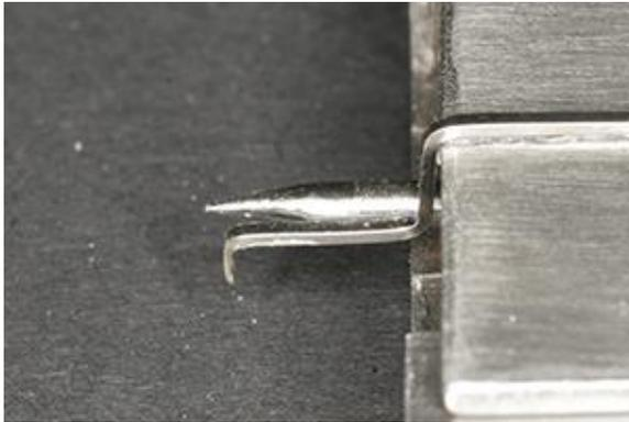
Fig. 4. Two tips placed on flat surface for zero setting.
