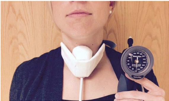
**FIGURE 1** Swallow Resistance Exercise Device (sRED) consists of an inflatable bag housed in a rigid shell. The concave surface of the inflated bag rests on the thyroid cartilage and conforms to the surface of the larynx, restricting the anterosuperior excursion of the hyolaryngeal complex
