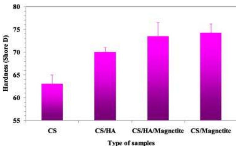
**Fig. 7.** The results of hardness test on the CS, CS/HA, CS/HA/magnetite, and CS/magnetite samples.
