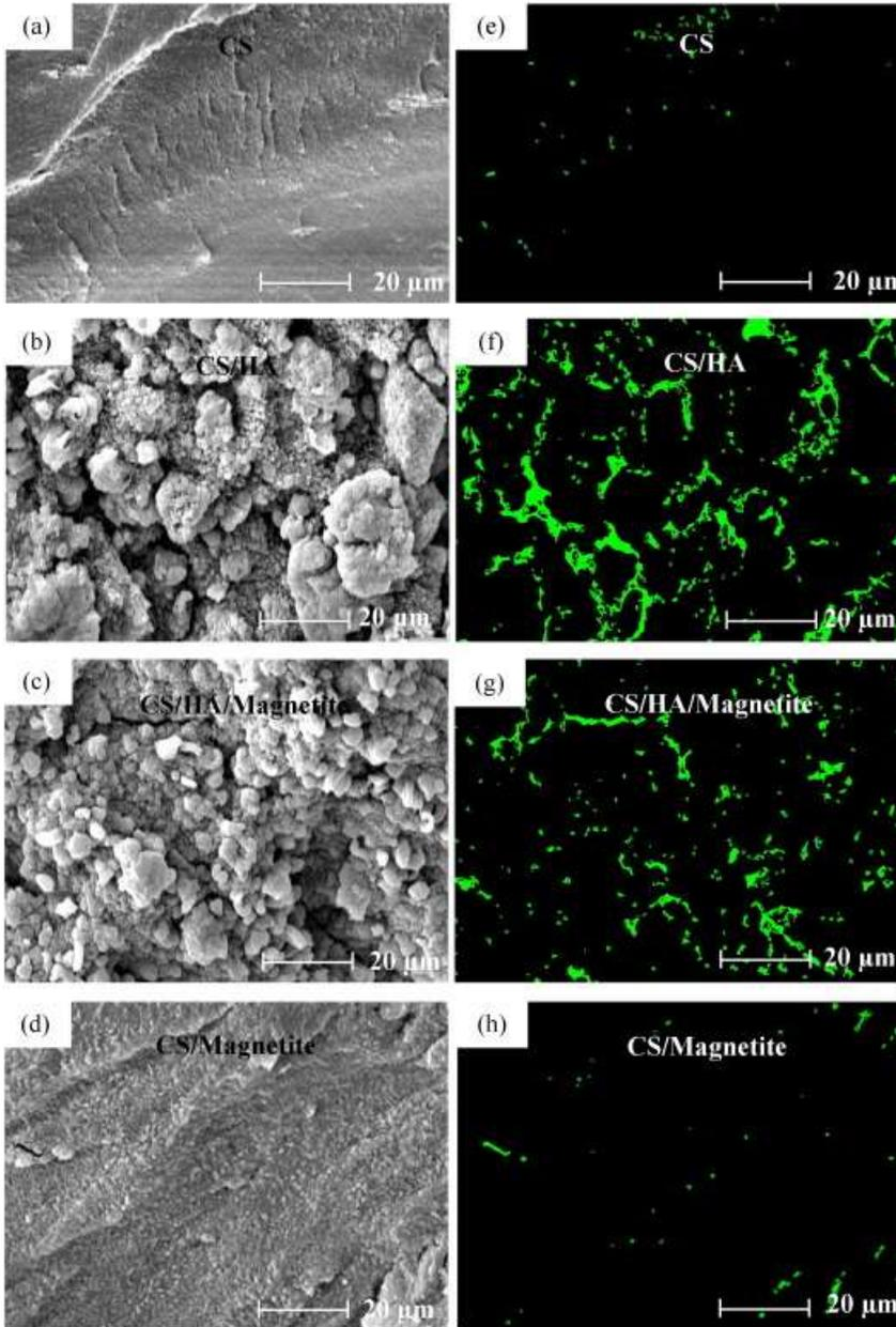
**Fig. 4.** SEM micrographs (a, b, c, d) and confocal images (e, f, g, h) from the cross-sectional view of CS (a), CS/HA (b), CS/HA/magnetite (c), and CS/magnetite (d) indicating the cracks and porosities in the fracture surface of samples after bending test.
