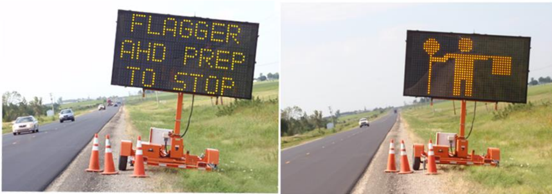
Figure 2. Text-graphic PCMS with the Flagger Graphic (from Huang and Bai (2014) Figure 4, license obtained)
