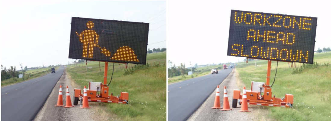
Figure 7. Text-graphic PCMS with Work Zone Graphic Alternative Two (from Huang and Bai (2014) Figure 10, license obtained)
