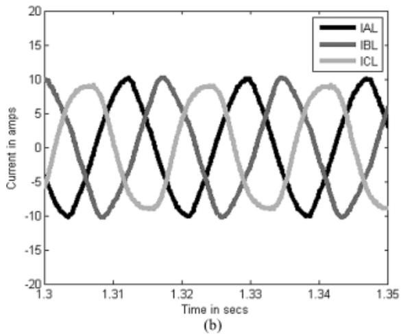
**Fig. 8** (a) Line currents, vector-control, when the introduced controller was deactivated for the faulty two-phase open-delta operation, operating at 120 rad/s. "Coupled Simulink/Flux2D model." (b) Line currents, open-loop, when the introduced controller was activated for the two-phase open-delta operation, operating at 120 rad/s. "Coupled Simulink/Flux2D model."
