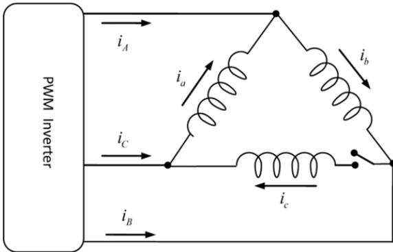
**Fig. 1.** Open-delta connection in stator windings.
