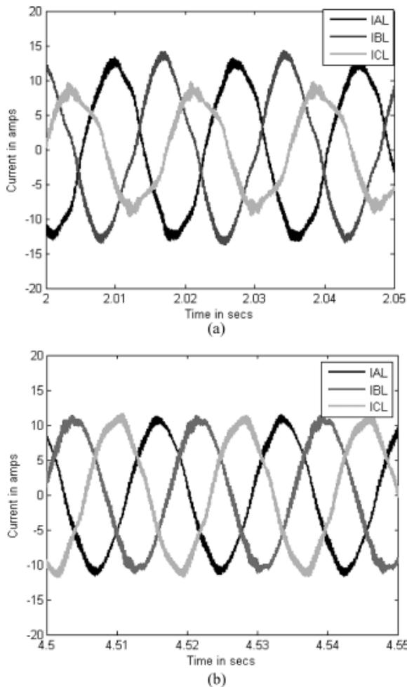
**Fig. 9** (a) Experimentally obtained line currents, vector-control, when the introduced controller was deactivated for the two-phase open-delta operation, operating at 120 rad/s. (b) Experimentally obtained line currents, vector-control, when the introduced controller was deactivated for the two-phase open-delta operation, operating at 120 rad/s.
