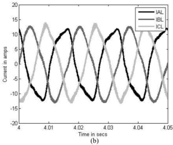
**Fig. 7** (a) Experimentally obtained line currents, open loop, when the introduced controller was deactivated for the two-phase open-delta operation, operating at 60 Hz. (b) Experimentally obtained line currents, open loop, when the introduced controller was activated for the two-phase open-delta operation, operating at 60 Hz.
