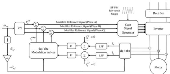
**Fig. 3.** Functional block diagram of the proposed algorithm for the case of scalar open-loop control motor-drive system.
