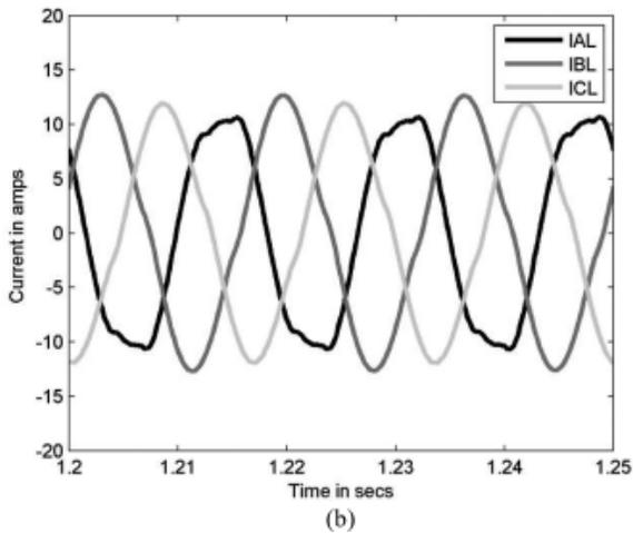
**Fig. 6** (a) Line currents, open loop, when the introduced controller was deactivated for the faulty two-phase open-delta operation, operating at 60 Hz. “Coupled Simulink/Flux2D model.” (b) Line currents, open loop, when the introduced controller was activated for the two-phase open-delta operation, operating at 60 Hz. “Coupled Simulink/Flux2D model.”
