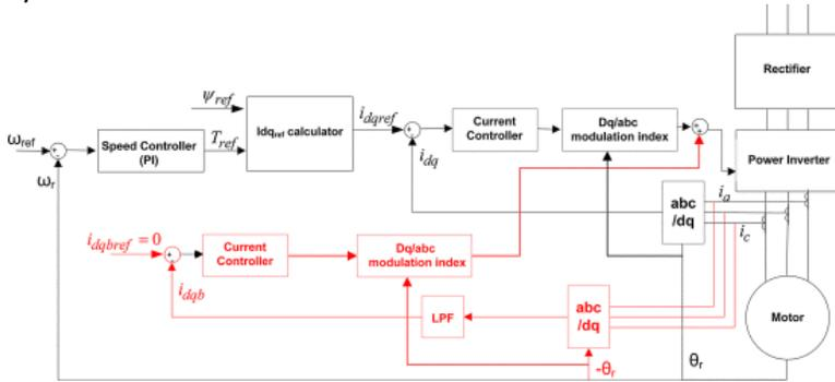
**Fig. 4.** Functional block diagram for the proposed algorithm for vector-control motor-drive systems.
