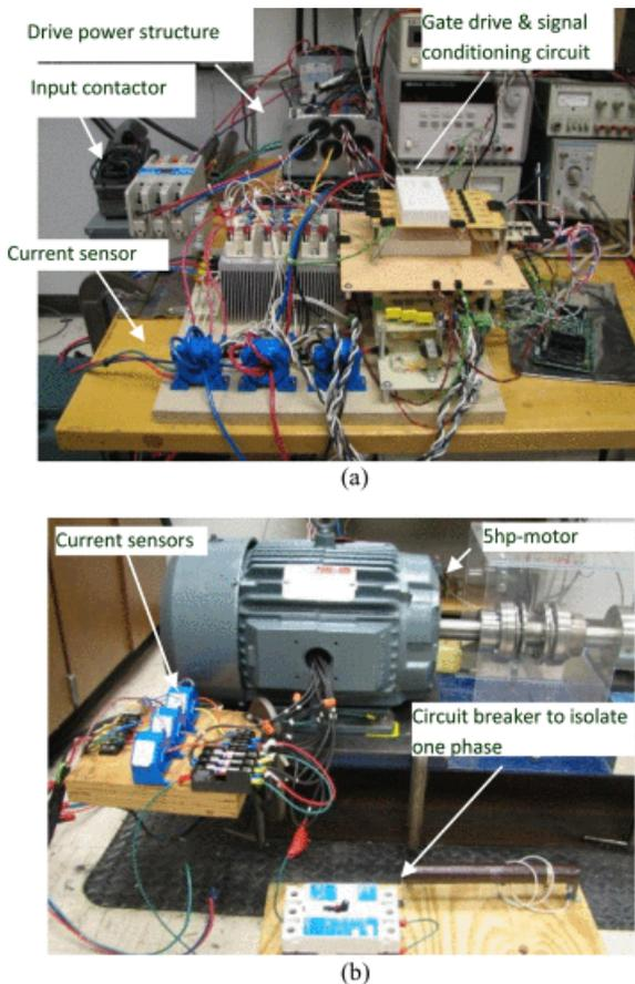
**Fig. 5** (a) Power converter utilized in the experimental testing. (b) Case study motor utilized in the experimental setup.
