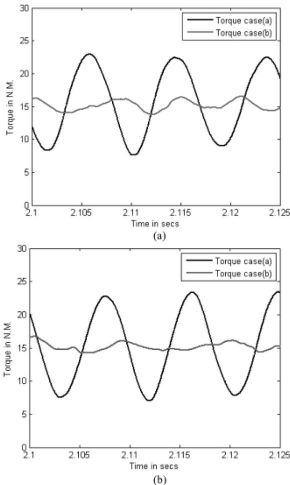
**Fig. 11** (a) Experimentally obtained output torque, open-loop for the two-phase open-delta operation, operating at 60 Hz. (b) Experimentally obtained output torque, vector-control for the two-phase open-delta operation, operating at 120 rad/s. Case (a) Introduced controller deactivated. Case (b) Introduced control activated.
