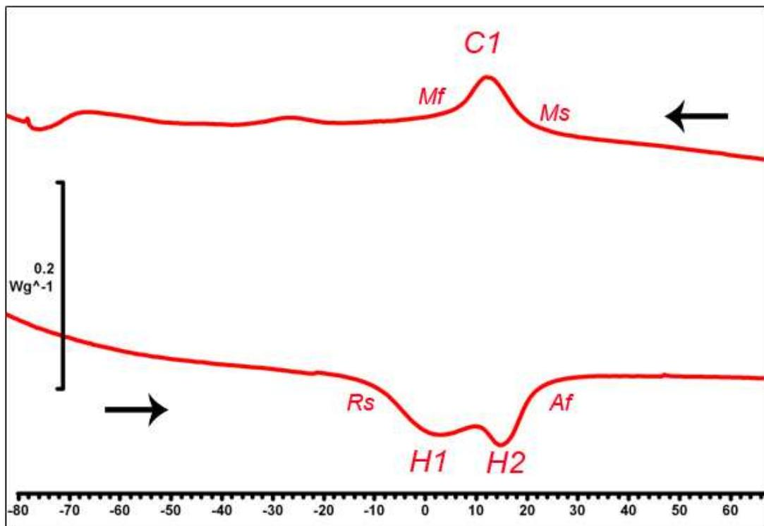
Figure 1: DSC thermogram for heating and cooling of wire samples.
