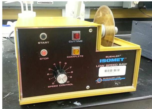
Figure 3: Water-cooled diamond saw (Buehler, Lake Bluff, IL).
