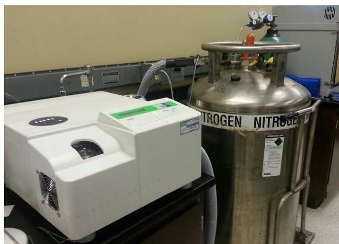
Figure 6: DSC equipment and liquid nitrogen.
