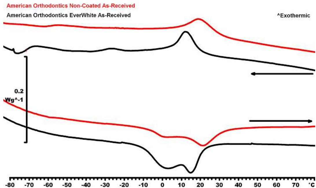
Figure 8: Thermograms of as-received American Orthodontics uncoated and EverWhite wires.
