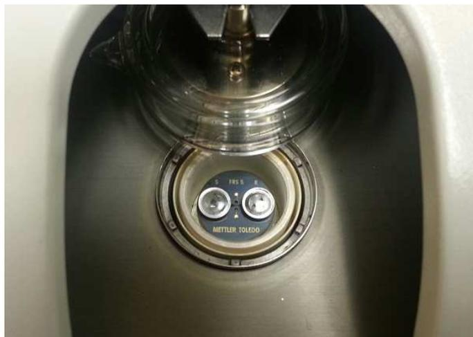
Figure 5: Aluminum crucibles on the sensor of the DSC. The crucible containing the wire sample is on the left and the blank reference crucible is on the right.
