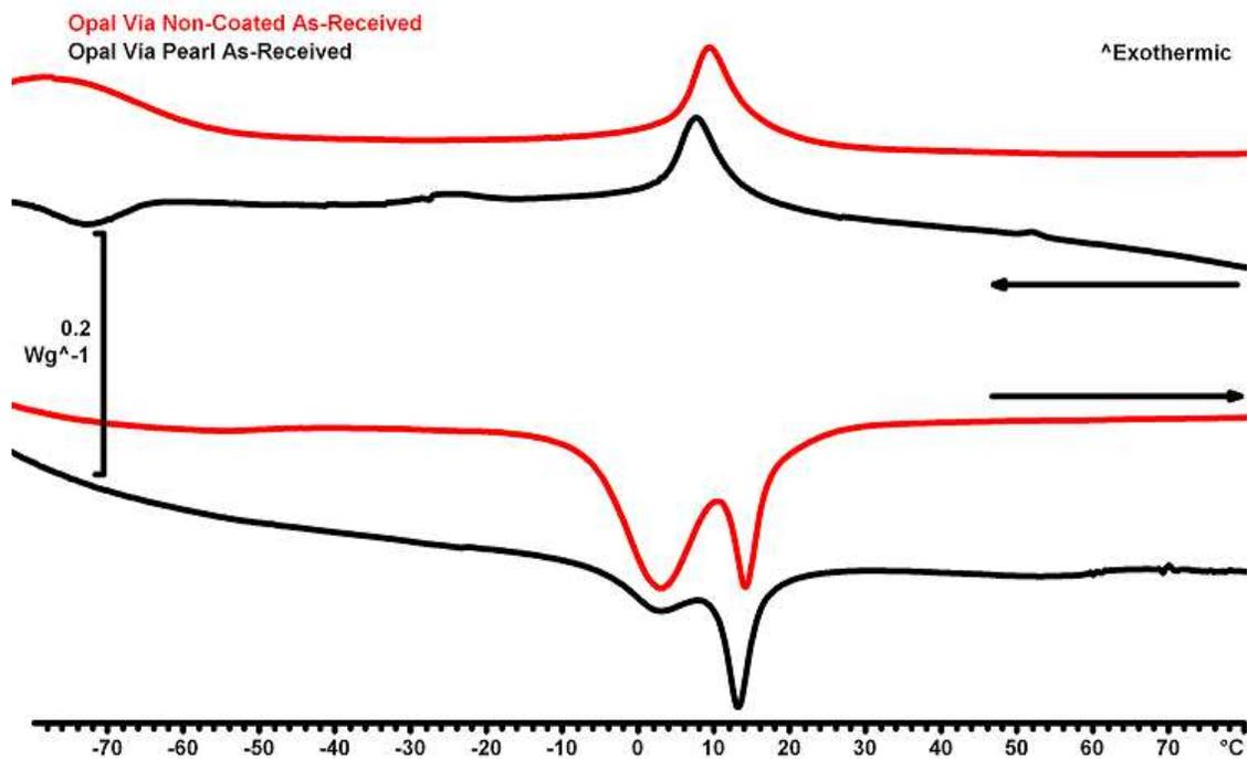
Figure 9: Thermograms of as-received Opal uncoated and esthetic Via Pearl wires.
