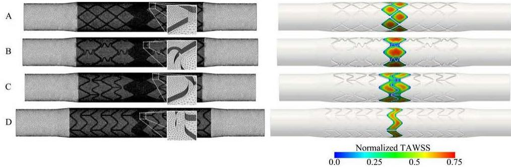
**Fig. 3.** (Left) Anisotropic meshes used for CFD. (Right) TAWSS depicted on the stent cells that are extracted and quantified during the optimization routine. TAWSS is shown normalized to the analytically computed value of TAWSS in an unstented portion of the vessel.
