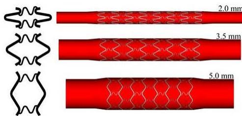
**Fig. 2.** Illustrations of the expanded geometry of single-stent cell (left) that were used to generate the three representative solids models of an idealized stented coronary (right). The vessel diameter depicted above each model corresponds to stent diameters of 2.2, 3.85, and 5.5 mm. The six crown configuration of stent B is depicted in each model.
