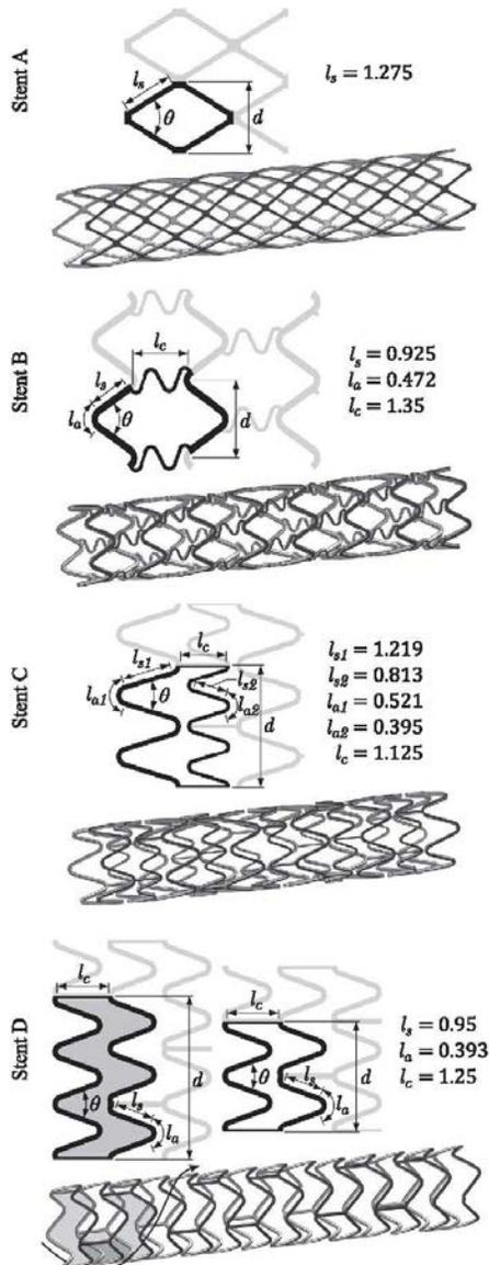
**Fig. 1.** Geometry of a single cell and related dimensions along with an expanded configuration of each stent design. All dimensions are given in millimeters. Each of the expanded stents shown has a diameter
