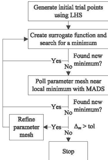
**Fig. 4.** Flowchart of the SMF optimization routine. The routine is initialized using LHS, and then uses search and MADS polling operations to converge on the optimal design parameter. The routine stops once a local minimum has been found and the resolution of the discrete parameter mesh  $\Delta_m$  has been refined beyond a user defined tolerance (tol).
