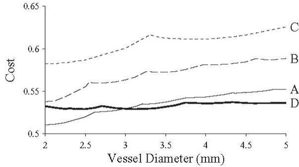
**Fig. 7.** Comparison of the least-cost curves of each stent design. The least-cost curve represents the best hemodynamic cost function value from all configurations of a given stent design for vessel diameters between 2.0 and 5.0 mm in diameter.
