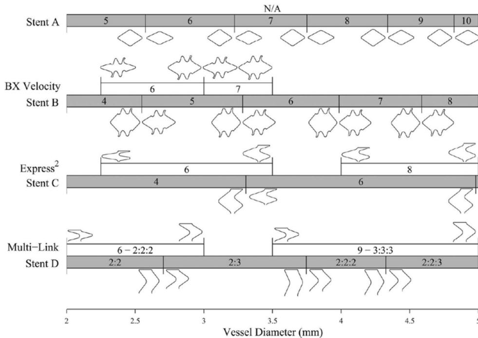
**Fig. 8.** Comparison of the vessel diameter range of commercially available stents with the hemodynamically optimal diameter range. The expanded geometry of a single circumferential crown corresponding to the minimum and maximum cell expansion of each range is also shown.
