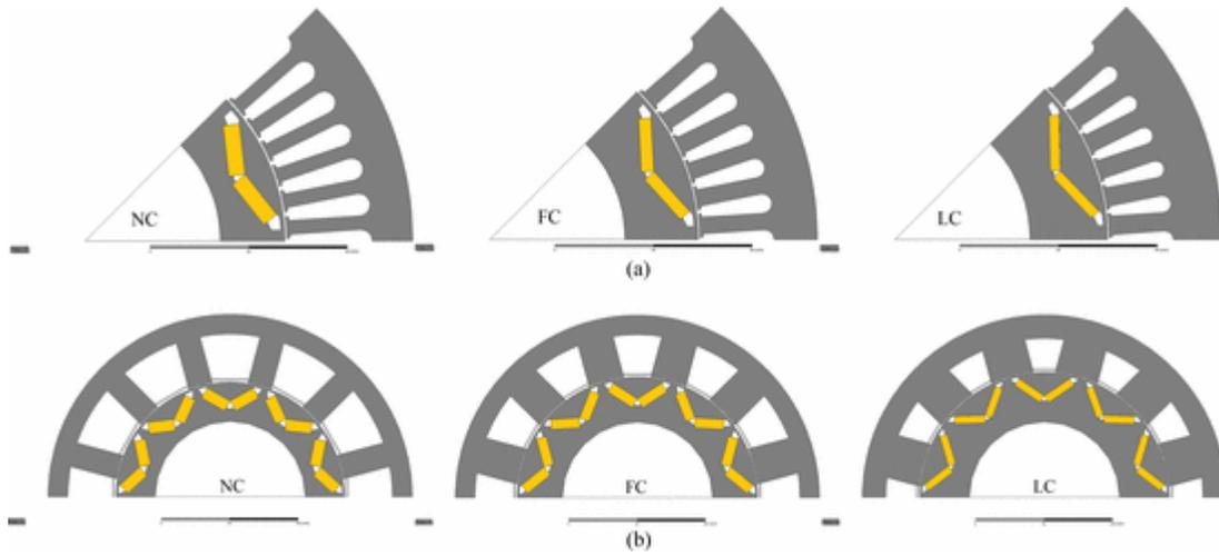
Fig. 5. Optimized cross sections derived based on the mean of the design variables in the 500 Pareto-optimal designs, see [Table III](#), for the three current density levels: (a) 48S8P, and (b) 12S10P machines.
