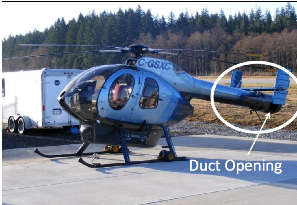
Figure 7. Shaftless Anti-torque System http://jetav.com/md-520n-specifications/
