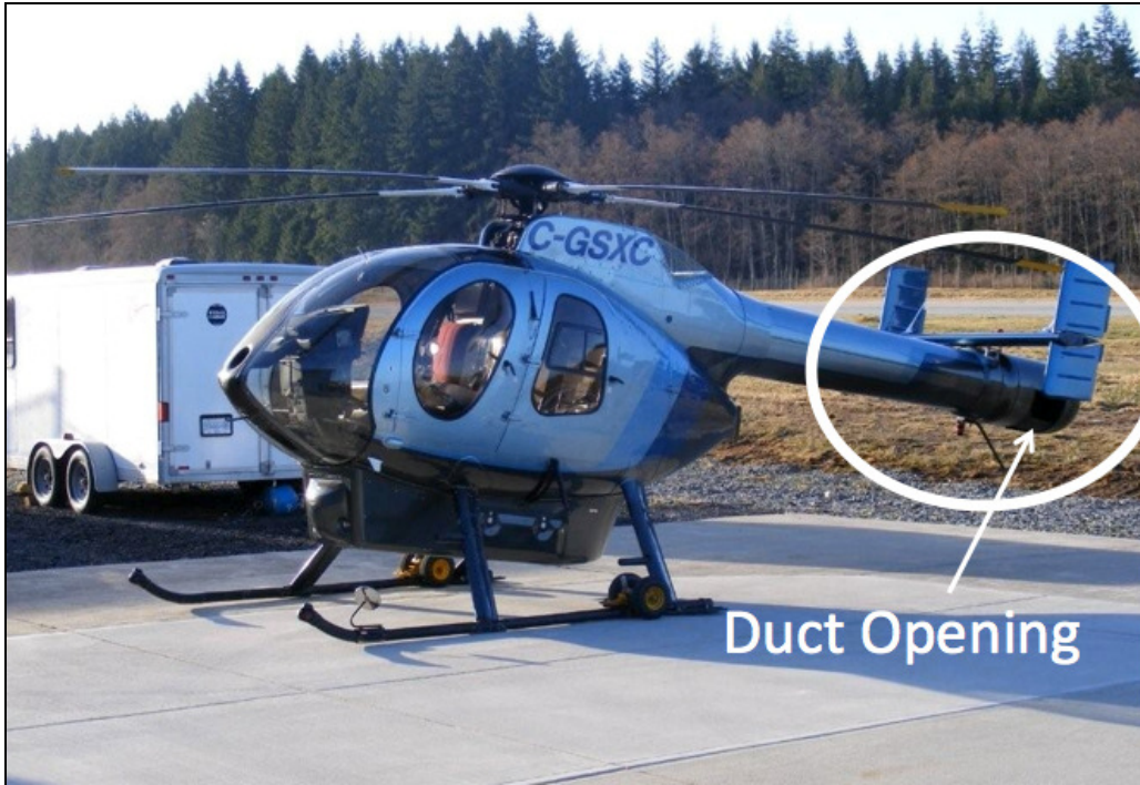
Figure 7. Shaftless Anti-torque System http://jetav.com/md-520n-specifications/
