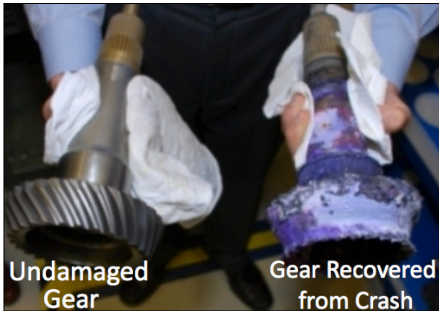
Figure 9. Failed Gear Comparison
