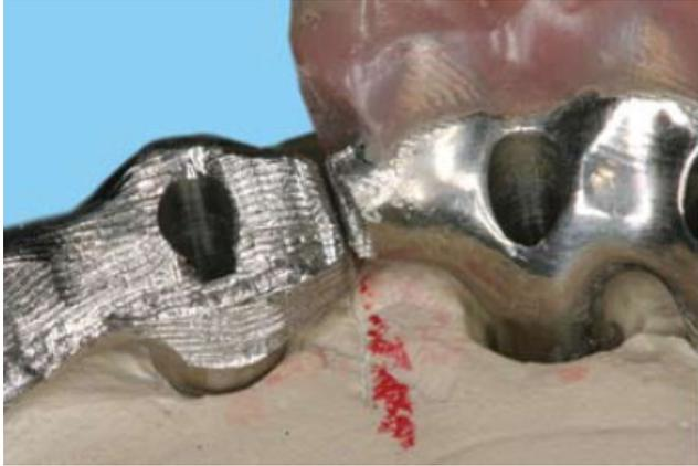
Fig. 5. Assembled existing and new framework sections to be laser welded.
