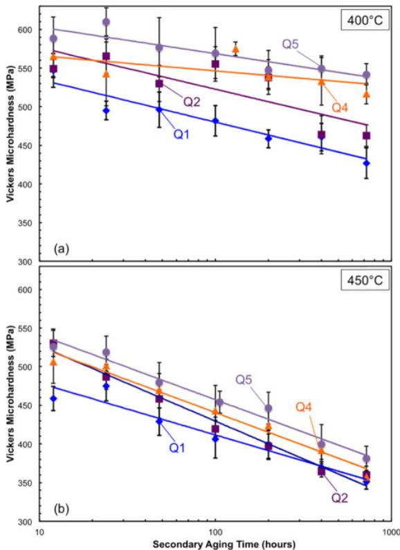
Fig. 2. Vickers [microhardness](#) (MPa) plots versus secondary aging time (hours) displaying its evolution for alloys Q1 (unmodified), Q2 (V-modified), Q4 (Nb-modified), and Q5 (Ta-modified) during double-aging with a primary step at 350 °C for 16 h, followed by secondary steps at: (a) 400 °C; and (b) 450 °C for times between 12 and 720 h.
