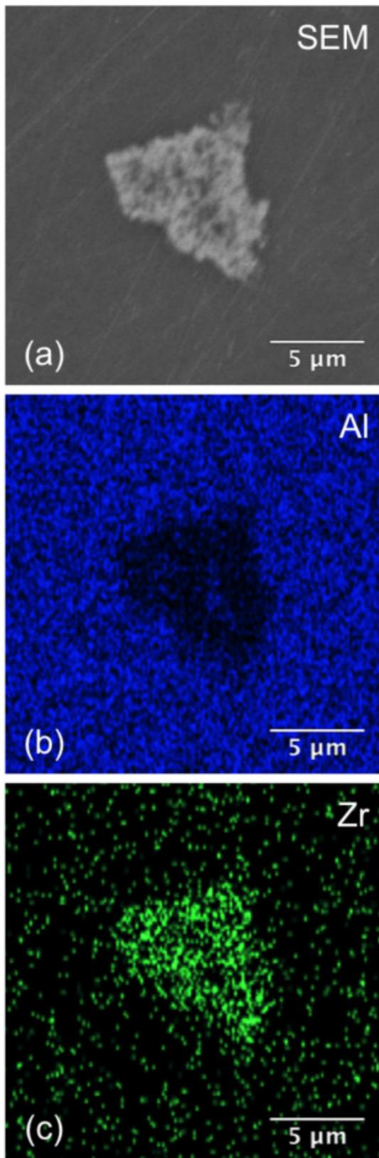
Fig. 1. (a) [Scanning electron microscopy](#) (SEM) image showing a primary  $\text{Al}_3\text{Zr}$  precipitate in the as-cast alloy Q4. Energy dispersive [X-ray spectroscopy](#) (EDS) maps displaying the distributions of (b) Al and (c) Zr.
