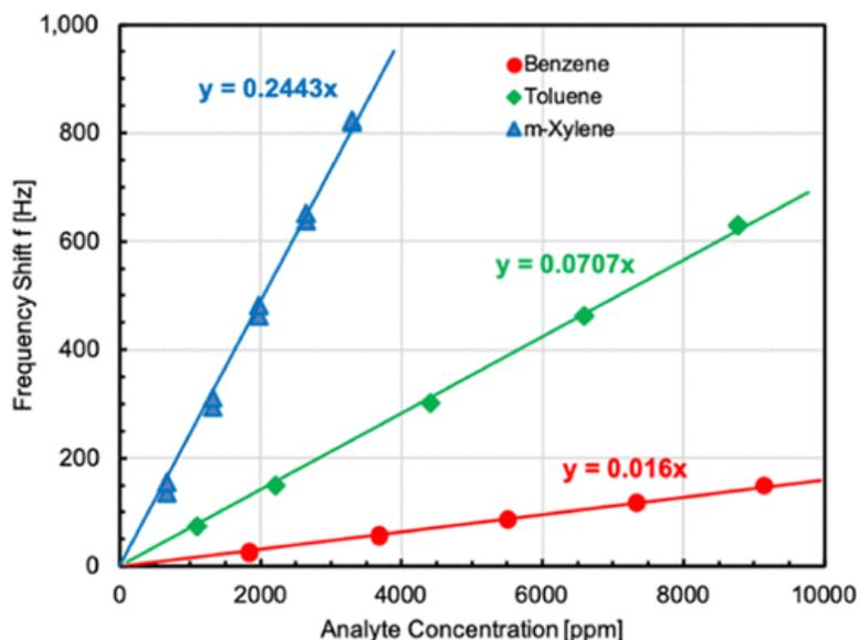
Figure 9. Sensitivity curves showing the absolute value of the measured steady-state frequency change for the F200A hammerhead resonator coated with 1.5  $\mu\text{m}$  PIB as a function of *m*-xylene, toluene, and benzene concentrations.
