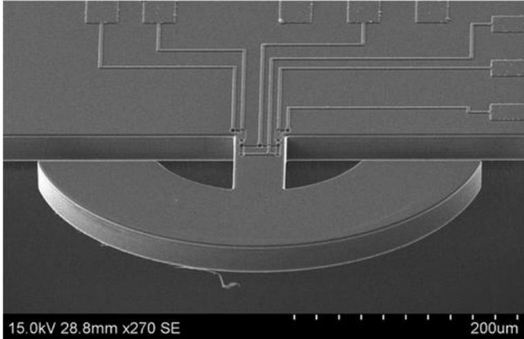
Figure 4. SEM micrograph of a F200A hammerhead device with a 45  $\mu\text{m}$  wide and 100  $\mu\text{m}$  long support cantilever and a semicircular annulus with an outer radius of 200  $\mu\text{m}$ . The piezoresistive Wheatstone bridge and thermal excitation resistors can be seen at the base of the device.
