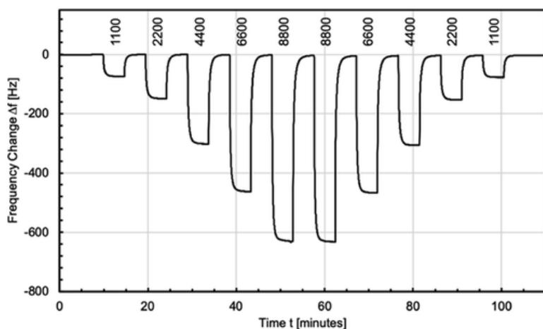
Figure 8. Sample gas measurement exposing a F200A hammerhead resonator (20  $\mu\text{m}$  silicon thickness) coated with 1.5  $\mu\text{m}$  PIB to different toluene concentrations. Analyte concentrations in ppm are shown in the graph.
