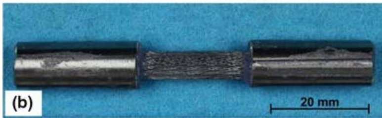
Fig. 3 Tensile test sample with grips: (a) cross section of the grip with steel core (marked with “C”) and half tubes (marked with “T”) and (b) sample showing gage and grip sections
