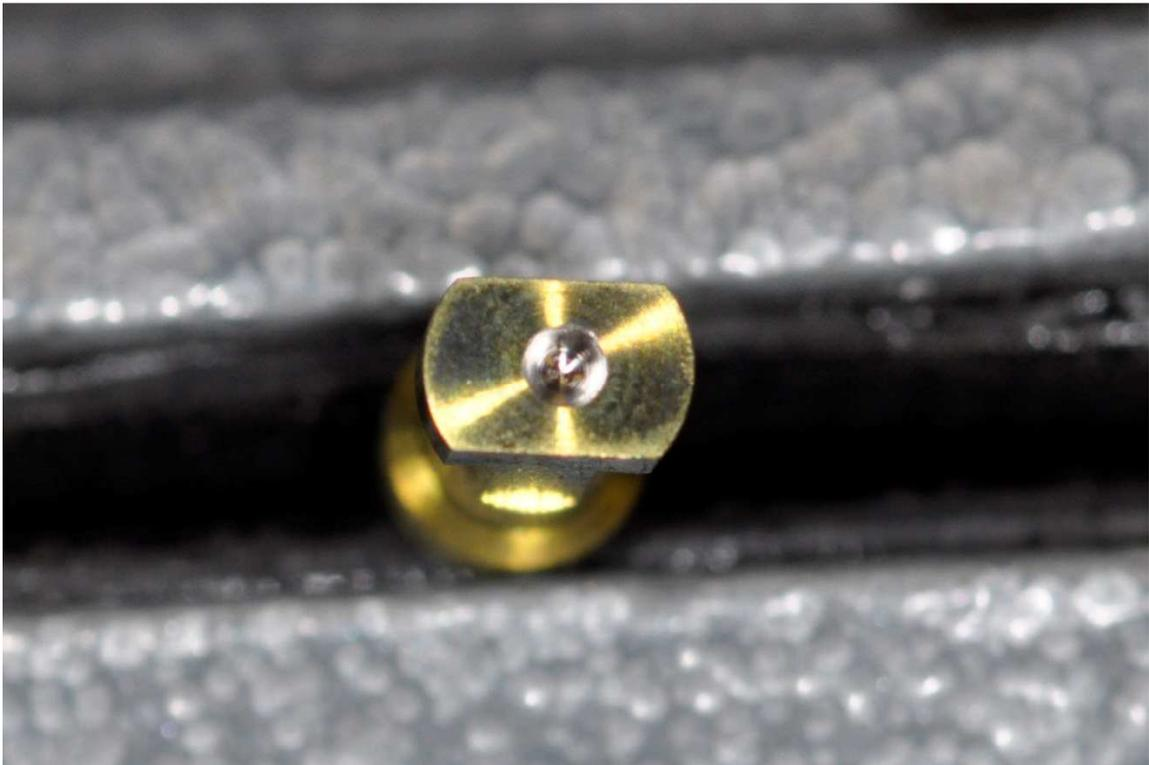
Figure 8: Machined dimple.
