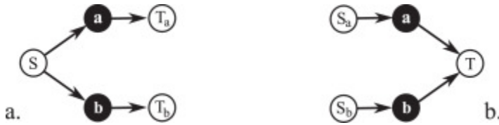
Fig. 5. Bifurcation branch roadmap of a task path crossing a single coregular value. a) The roadmap of a task starting with 1 self-motion manifold and terminating with 2 self-motion manifolds. b) The roadmap of a task starting with 2 self-motion manifolds and terminating with 1 self-motion manifold.
