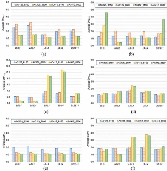
**Figure 3.** Ratio of the allowable number of repetitions to failure comparing DTA with NG-WBT for thick pavement structures: (a)  $DW$  for bottom-up cracking; (b)  $DW$  for top-down cracking due to tensile strain; (c)  $DW$  for top-down cracking due to shear strain; (d)  $DW$  for AC rutting; (e)  $DW$  for subgrade rutting; (f)  $CDW$  considering all five distresses.
