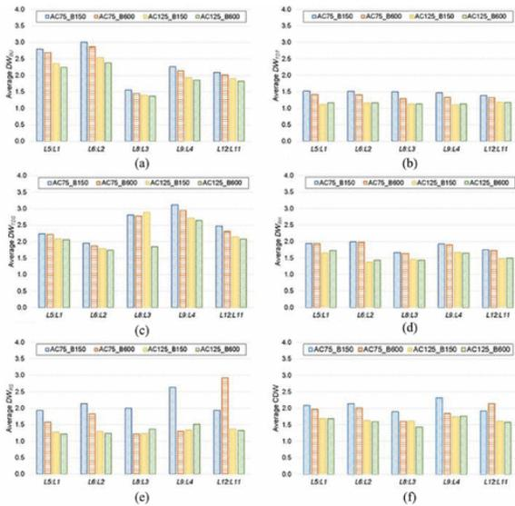
**Figure 2.** Ratio of the allowable number of repetitions to failure comparing DTA to NG-WBT for thin pavement structures: (a)  $DW$  for bottom-up cracking; (b)  $DW$  for top-down cracking due to tensile strain; (c)  $DW$  for top-down cracking due to shear strain; (d)  $DW$  for AC rutting; (e)  $DW$  for subgrade rutting; (f) CDW considering all five distresses.
