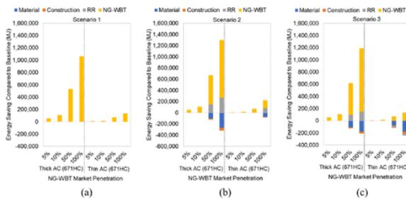
**Figure 7.** Net energy saving of using NG-WBT for (a) Scenario I, (b) Scenario II, and (c) Scenario III (33).
