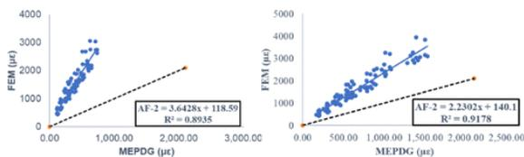
**Figure 4.** Maximum compressive strain within base for strong and weak base layers, respectively.
