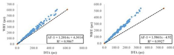
**Figure 5.** Maximum tensile strain at the bottom of the AC along the longitudinal and transverse direction, respectively.
