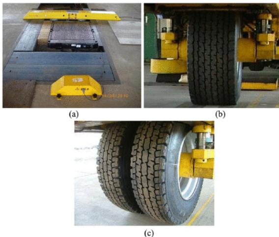
**Figure 1.** Tested tires and stress-in-motion system: (a) stress-in-motion systems; (b) new-generation wide-base tire 445/R22.4; (c) dual-tire assembly 275/80R22.5
