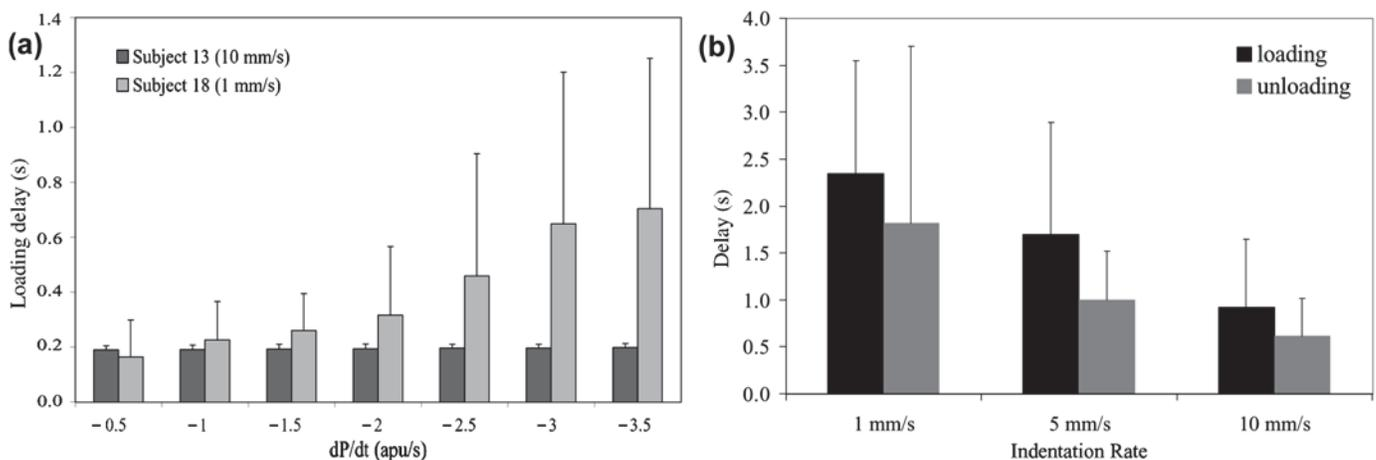
**Figure 7.** (a) Dependence of mean loading delay on perfusion slope threshold for 10 loading cycles for Subjects 13 (10 mm/s, black) and 18 (1 mm/s, gray). (b) Loading (and unloading or recovery) delays were computed with maximum cross-correlation coefficient.
