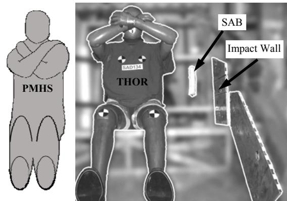
Figure 2. Occupant surrogate positioning in sled buck. Impact wall and seat-mounted SAB are indicated. Door-mounted SAB was positioned at thorax level within impact wall.
