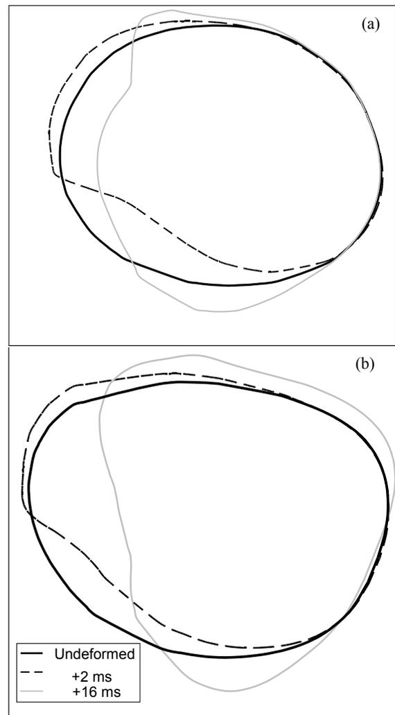
Figure 12. Chestband contours at level demonstrating posterolateral deformation of (a) THOR and (b) PMHS occupant surrogates with OOP seat-mounted SAB deployment.
