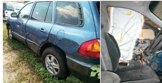
Figure 7. Case 4 vehicle damage and SAB.
