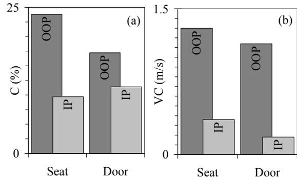
Figure 11. Peak lateral biomechanical metrics of (a) compression and (b) viscous criterion calculated in THOR deformation for seat- and door-mounted SABs. Out-of-position (OOP) and in-position (IP) scenarios are indicated.
