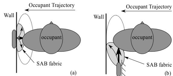
Figure 9. Deployment scenario for sled tests with (a) door-mounted and (b) seat-mounted SAB.
