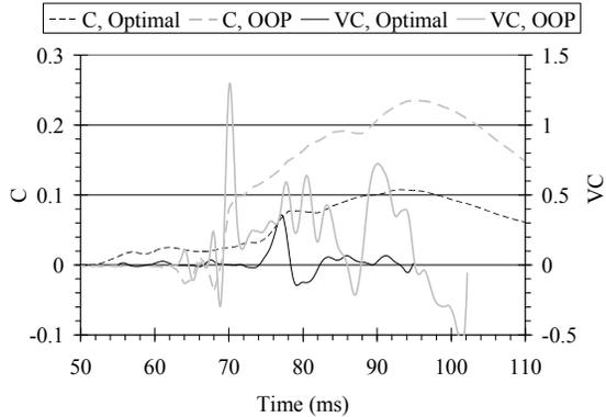
Figure 10. Lateral biomechanical metrics of compression and viscous criterion in time domain for THOR seat-mounted SAB in optimal and OOP scenario.
