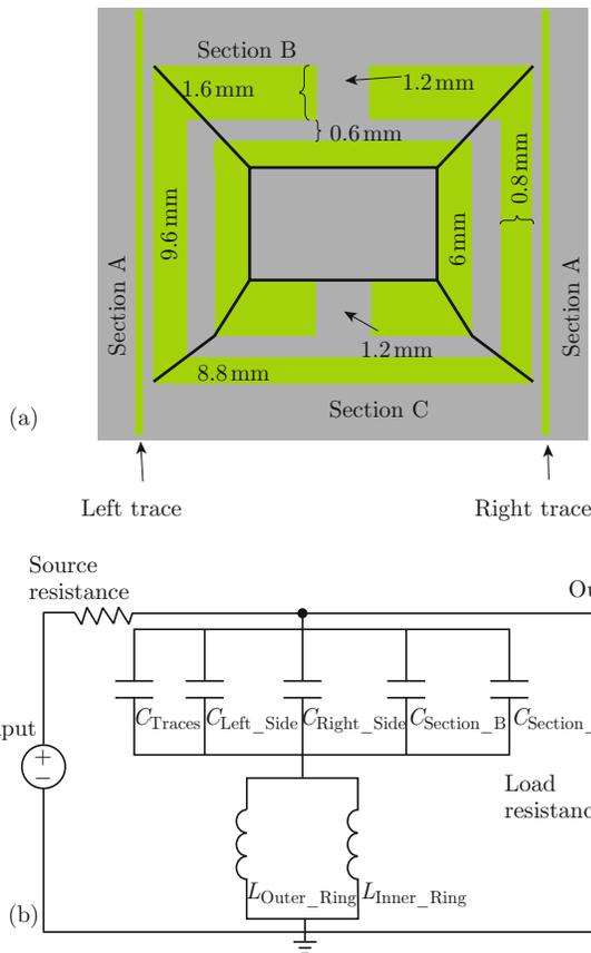
Fig. 1 (a) Baseline meta-atom indicating sections and dimensions. (b) The equivalent LC circuit model representing the meta-atom design.
