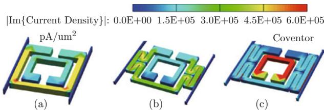
Fig. 4 CoventorWare<sup>®</sup> plots showing magnitude of imaginary current density incident on the (a) Baseline, (b) Loop A and (c) Loop B versions of the meta-atom designs.
