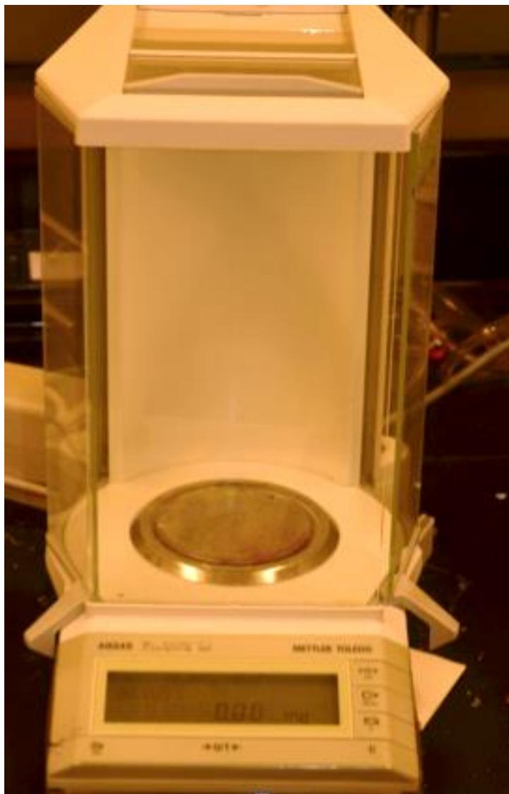
**Figure 3:** Scale used to measure wire segments
