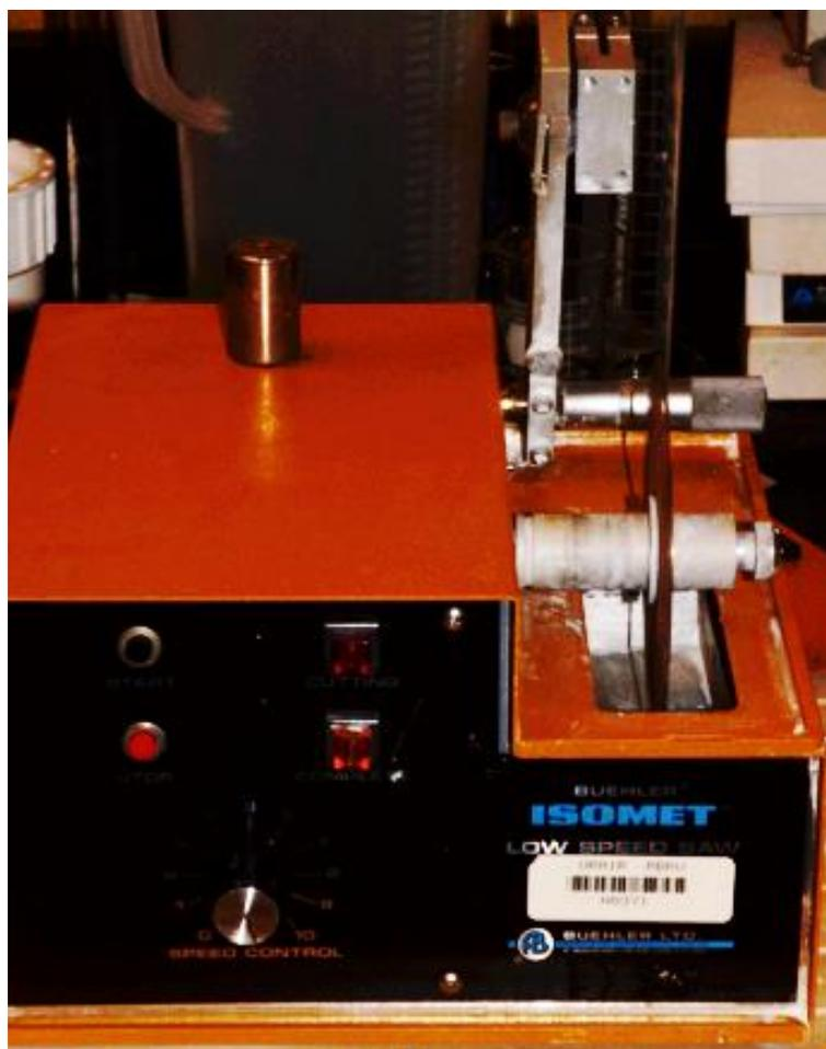
**Figure 2:** Isomet Diamond Saw used to section wires
