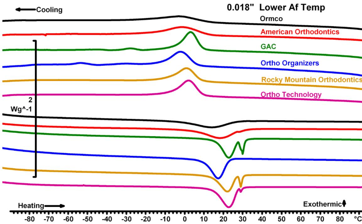
Figure 8: Thermogram for 0.018” wires with Af of 27°C
