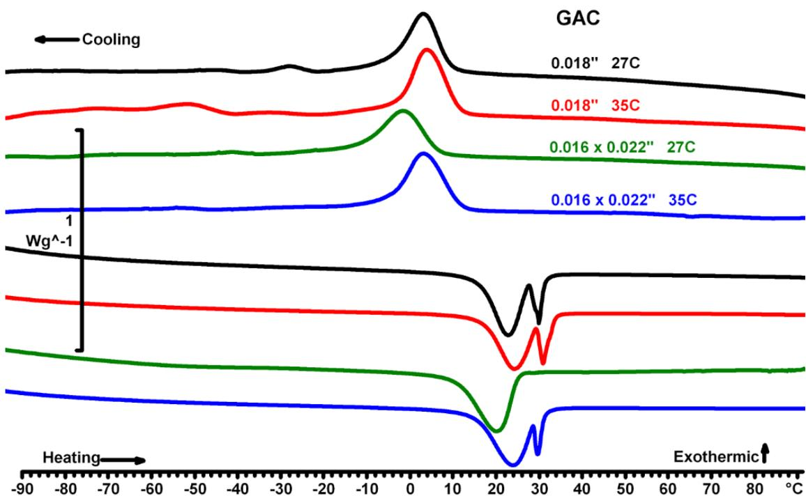
Figure 14: Thermogram for all variants of GAC CuNiTi wires
