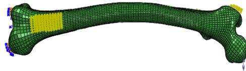
**Figure 1:** FE model of OI type I femur.
