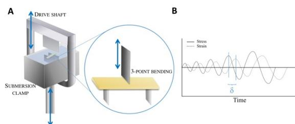
Fig. 1. Dynamic mechanical analysis. A. Illustration of the 3-point bending submersion clamp. A dynamic load is applied by the drive shaft in the middle of the specimen. B. Depiction of the phase angle  $\delta$  or phase shift formed between the deformation and the response of a viscoelastic material vs.
