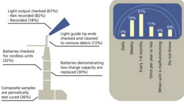
Frequency of checking light output
