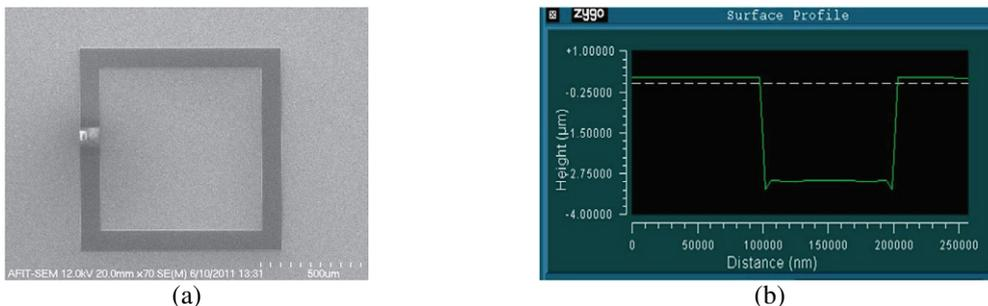
Figure 1 (a) Scanning electron microscope (SEM) image of a pre-bonded 1mm x 1mm SU-8 rectangular bonding ring (150µm-wide) test structure, (b) IFM surface profile of the SU-8 ring showing  $\sim 3 \mu\text{m}$  step height of the SU-8 rectangular ring.
