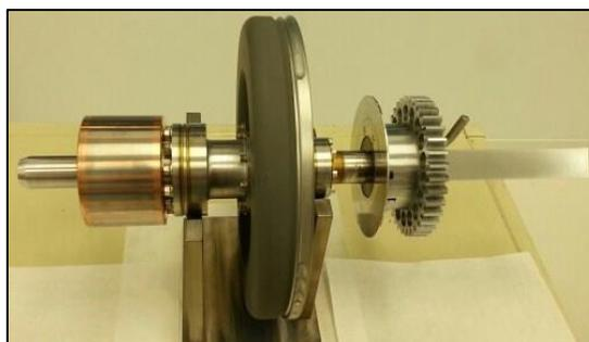
Figure 24: An anode which has the collets attached and is ready for placement into the machine.
