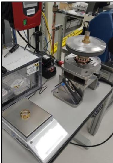
Figure 59: Sleeve seal was removed and weighed on the scale to determine the amount of Ga in the traps.
