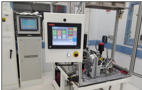
Figure 3: The balance machine which performs the balancing operation.
