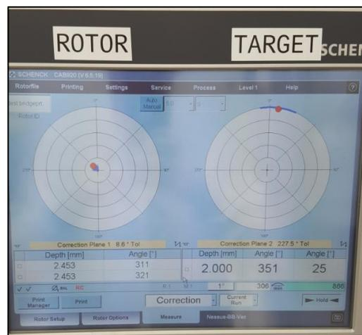
Figure 31: This screen outputs where and how the correction will take place based on the unbalance. This information is sent to the HMI, Figure 32, so that the operator can begin the material removal process.
