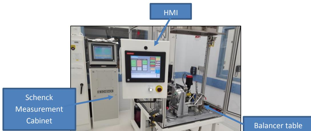
Figure 22: Balancer system comprised of Schenck Measurement Cabinet, HMI or Human Machine Interface, and balancer table.
