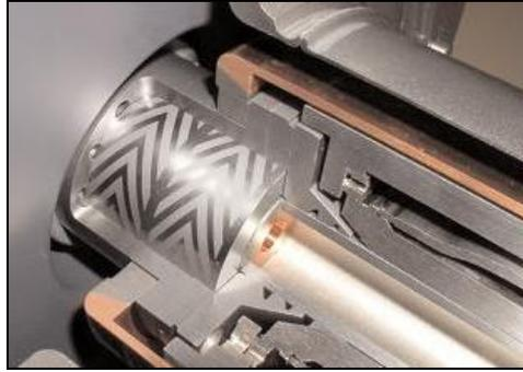
Figure 14: Example of cut away from a SGB insert showing two radial bearings of a liquid metal lubricated SGB [11].
