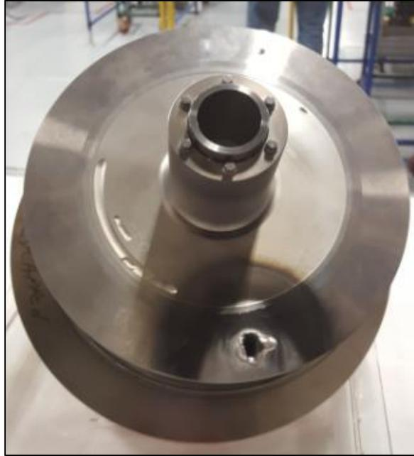
Figure 8: Example of a track melt on an x-ray tube anode.
