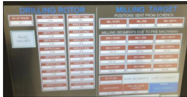
Figure 32: HMI screen showing the depths and degree of the cuts to be made for the rotor and target planes.
