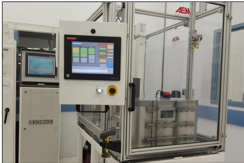
Figure 26: Balance machine with vacuum chamber closed with the anode inside.
