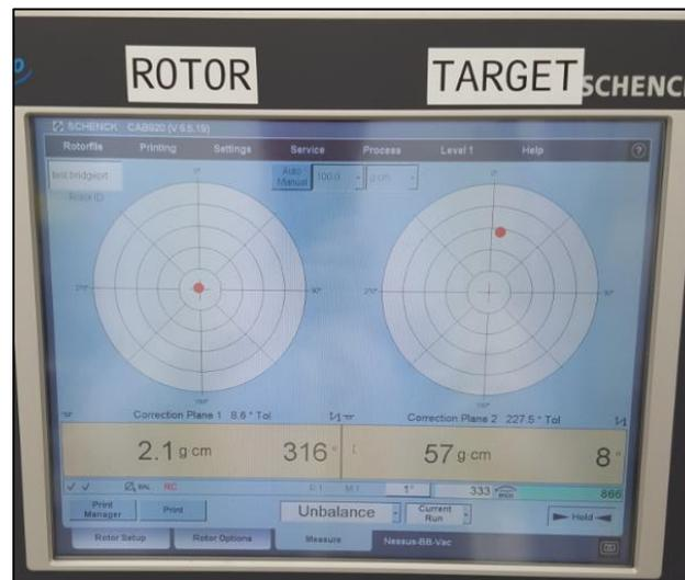
Figure 30: Example of the Schenck output that tells where and what the unbalance is after a balance measurement run.
