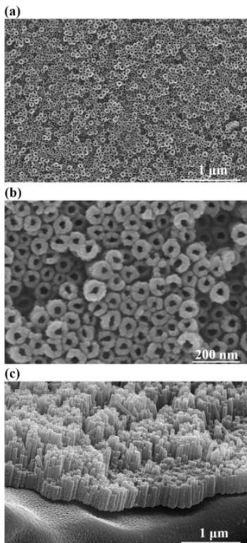
Fig. 2. FESEM micrograph of the sample subjected to the sequence of anodization, sonication and annealing from top views in two magnifications (a, b) and a tilted view (c).
