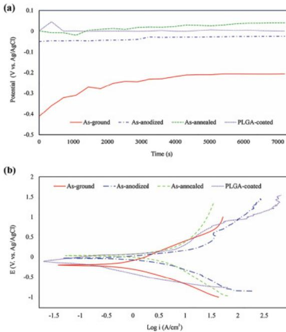
Fig. 7. Open circuit potential (a) and potentiodynamic polarization (b) curves of the samples.
