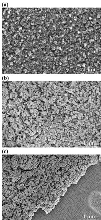
Fig. 1. FESEM micrograph of the samples processed by anodization (a), anodization followed by sonication for 5 min (b) and anodization followed by sonication for 10 min (c).
