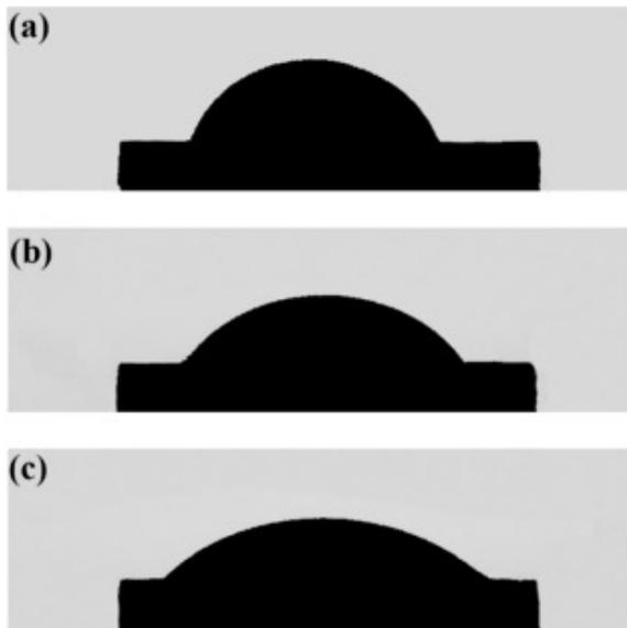
Fig. 4. Side-view macrograph of water drops on the as-ground (a), as-anodized (b) and annealed (c) samples.
