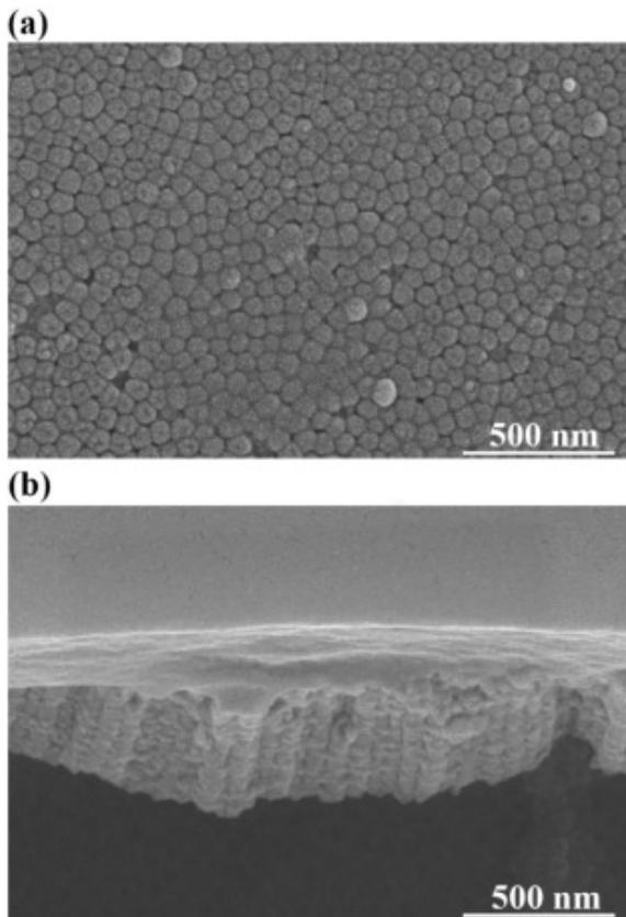
Fig. 3. FESEM micrograph of the NTs loaded with vancomycin from a top view (a) and coated with PLGA from a tilted view (b).
