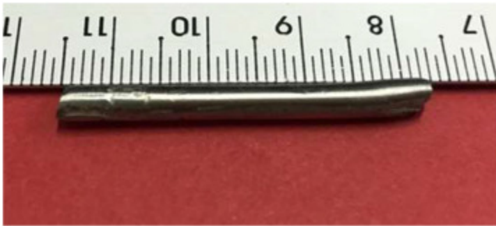
Fig. 3. Typical of ASTM F2581 alloy produced utilizing the BAE method.
