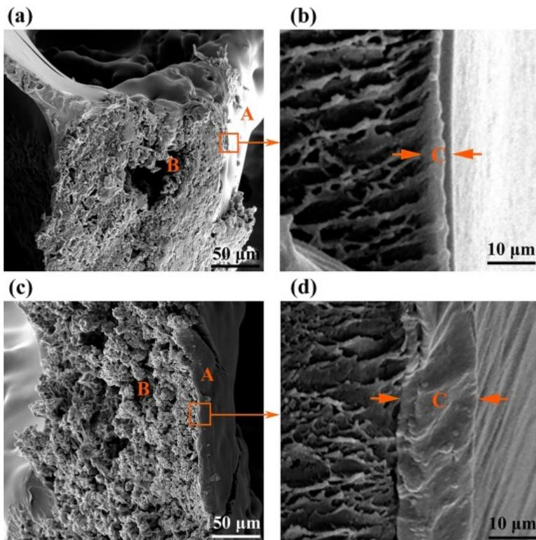
Fig. 3. Cross-sectional FESEM micrographs of the 5% (a, b) and 10% (c, d) PLGA-coated bredigite struts, where A, B and C represent the PLGA coating surface, bredigite strut cross section and PLGA coating cross section, respectively.
