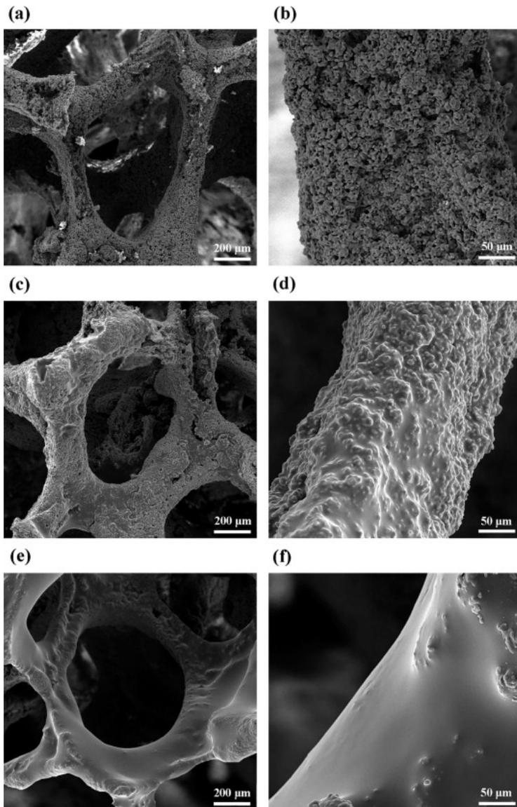
Fig. 2. FESEM micrographs of the bare (a, b), 5% PLGA-coated (c, d) and 10% PLGA-coated (e, f) bredigite scaffolds in two magnifications.
