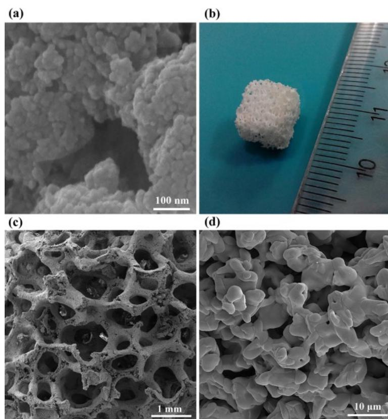
Fig. 1. FESEM micrograph of the sol-gel derived powder calcined at 700 °C (a), macrograph of the scaffold sintered at 1350 °C (b) and FESEM micrographs of the sintered scaffold in two magnifications (c, d).
