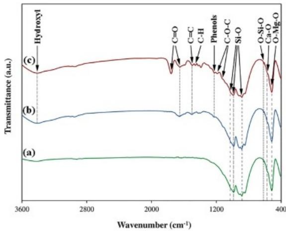
Fig. 4. FTIR spectra of the bare vancomycin-free (a), bare vancomycin-loaded (b) and PLGA-coated vancomycin-loaded (c) bredigite scaffolds.
