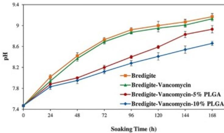
Fig. 6. pH variations of the SBF in contact with the different scaffolds.
