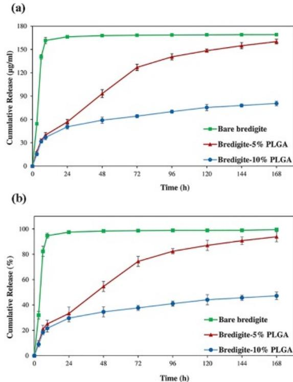
Fig. 5. Concentration (a) and percentage (b) of vancomycin released from the different scaffolds.
