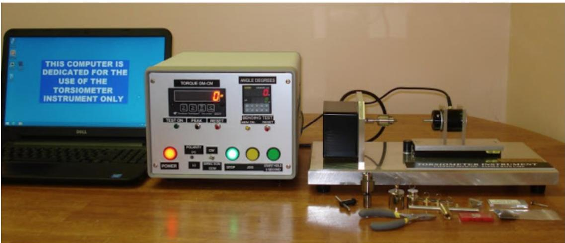
Figure 2. NiTi file set up for bending test in a torsionmeter
