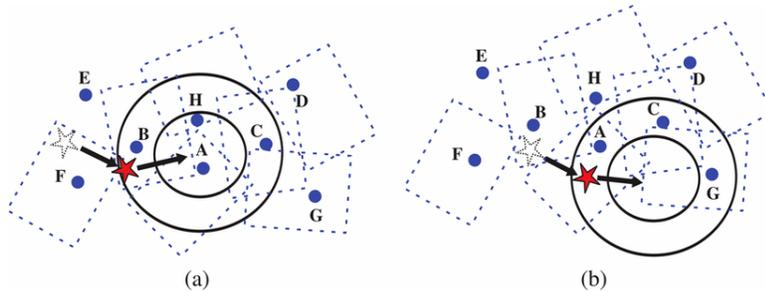
**Figure 1:** A depiction of a WCN engaged in tracking a moving object at two subsequent time instants. The dotted rectangles represent the sensing field of nodes. The red star indicates the object of interest and
