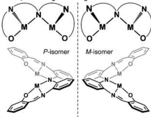
**Figure 4.** Illustration of the two possible orientations of the  $C_2$ -symmetric  $L^{N3O2}$  ligand in complexes **1–6**. The designations of the atropisomers (*M* and *P*) were based on rules developed for binaphthyl systems.
