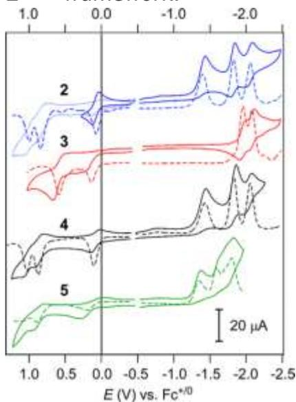
**Figure 7.** Cyclic voltammograms (solid lines) of complexes **2–5** collected in MeCN with 0.1 M  $(\text{NBu}_4)\text{PF}_6$  as the supporting electrolyte. Corresponding square-wave voltammograms are indicated by the dashed lines. All scan rates were 100 mV/s. Data
