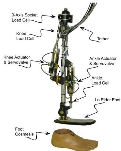
Figure 2.12: Knee and Ankle Prosthesis with Major Components [41]
