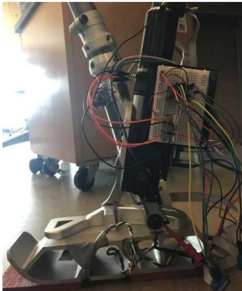
Figure 6.2: Side View of Marquette Prosthesis II with Hardware Attached
