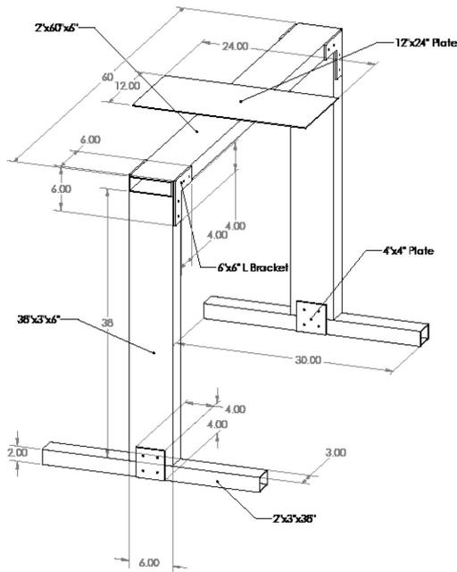
**Fig. 1.** Drawing made by an MU engineering student to communicate a proposed design concept for a movable stand to hold a hand ergometer over a patient's bed to allow the patient to exercise while lying flat on the bed. This drawing was generated in early December, just prior to the start of the MU/MIAD collaboration in January.
