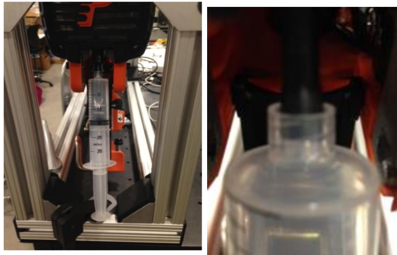
Figure 9. (a, left) Dosing syringe attached to combustion chamber. (b, right) “Close up” view of the connection syringe-to-tool connection.
