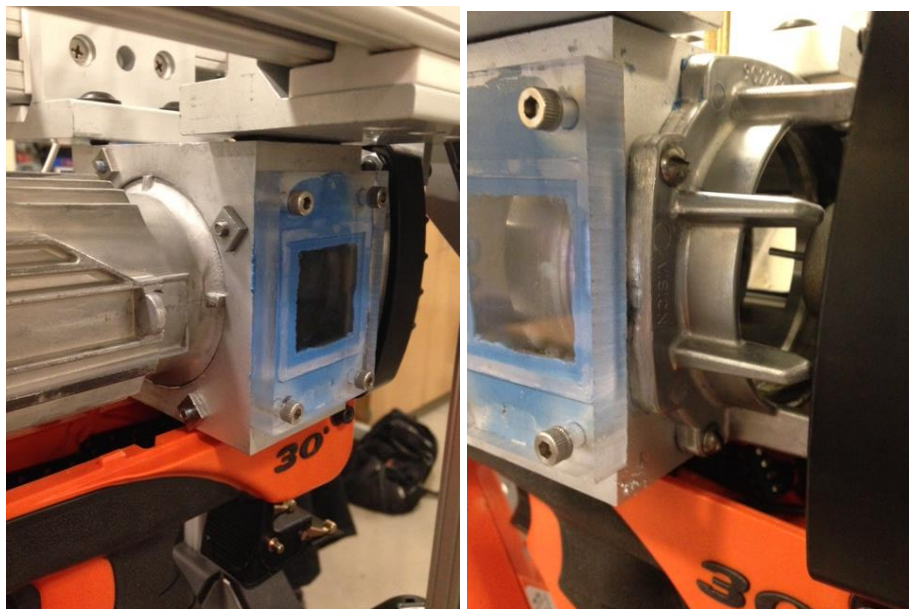
Figure 7. Photographs of the mounted, optically-accessible combustion chamber. (a, left) Depiction of the new chamber sealing with the current piston cylinder. (b, right) Depiction of the bolted connection between the original tool sealing component and the new chamber.
