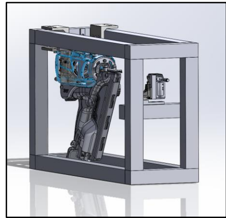
Figure 5. CAD model of test stand.
