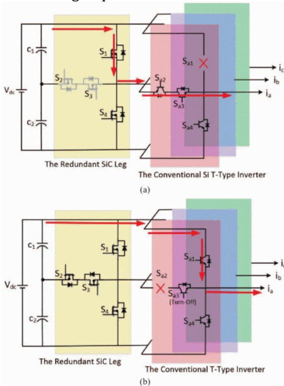
**Fig. 3** Current flow during fault-tolerant operation when (a) IGBT  $S_{a1}$  has an open-circuit fault (b) IGBT  $S_{a2}$  has an open-circuit fault (the devices in grey color refer to turn-off state).
