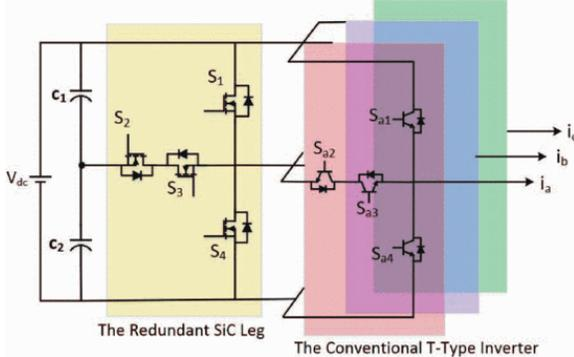
Fig. 2 The proposed fault-tolerant three-level T-type inverter topology.
