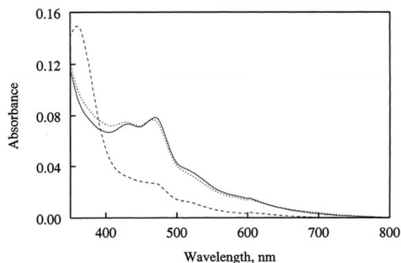
Figure 5 Thin-layer spectroelectrochemical oxidation of **1a** in DMF. Concentration of **1a** = 1.7 mM. Solid line: -0.60 V. Dashed line: +0.20 V. Dotted line: -0.80 V after oxidation at +0.20 V. All potentials vs Ag/AgNO<sub>3</sub> in acetonitrile. Concentration of TBAP: 0.20 M.
