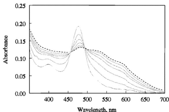
Figure 2 Thin-layer spectroelectrochemistry of **Ia** in methylene chloride. Concentration of **Ia** = 8 mM. Solid line: -0.60 V. Dotted lines: -0.90, -0.93, -0.96, -0.99, -1.02 V. Dashed line: -1.05 V vs Ag/AgNO<sub>3</sub> in acetonitrile. Concentration of TBAP: 0.20 M.
