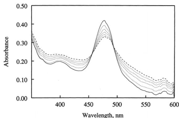
Figure 4 Thin-layer spectroelectrochemistry of **Ia** in methylene chloride obtained by stepping the potential to  $-1.05$  V. Solid line: initial spectrum. Dashed line: spectrum after 24 s. Dotted lines: intermediate spectra after 10, 15, 18, and 21 s. Concentration of **Ia** = 1.0 mM; concentration of TBAP = 0.10 M. Reference electrode: Ag/AgNO<sub>3</sub> in acetonitrile.
