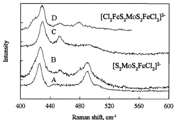
Figure 6 (A) Resonance Raman spectrum of **IIIa**. (B) Resonance Raman spectrum of the electrolysis product of **IIIa** at  $-1.25$  V. (C) Resonance Raman spectrum of **Ia** electrolyzed at  $-1.05$  V. (D) Resonance Raman spectrum of **Ia** electrolyzed at  $-1.05$  V, followed by addition of tetraphenylphosphonium chloride. All solutions in methylene chloride with 0.10 M TBAP. Reference electrode: Ag/AgNO<sub>3</sub> in acetonitrile.
