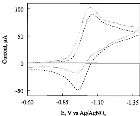
Figure 1 Cyclic voltammetry of **Ia** in methylene chloride in the presence and absence of chloride ion. Concentration of **Ia** = 2.1 mM. Solid line: 0 mM chloride. Dotted line: 8.0 mM tetrabutylphosphonium chloride. Scan rate: 100 mV/s, 0.10 M TBAP. Reference electrode: Ag/AgNO<sub>3</sub> in acetonitrile.
