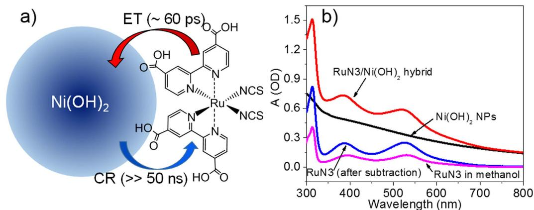
**Figure 1. The design of hybrid catalysts.** (a) Cartoon of charge separation and recombination dynamics in RuN3/Ni(OH)<sub>2</sub> hybrid. (b) UV-visible absorption spectra of Ni(OH)<sub>2</sub> NPs (black), RuN3/Ni(OH)<sub>2</sub> hybrid (red), RuN3 obtained after subtracting the spectrum of Ni(OH)<sub>2</sub> NPs from the spectrum of the hybrid (blue), and RuN3 in methanol (pink).
