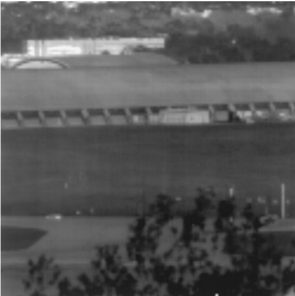
Fig. 5 Corrected version of the image of Fig. 2 obtained by use of the updated gain and offset. Note the improvement, which is due to recursion, in the correction compared with that of the image of Fig. 4 .
