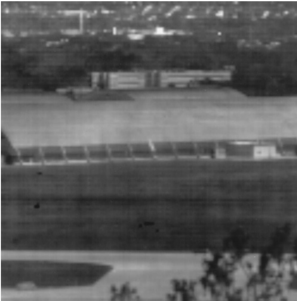
Fig. 9 Corrected version of the frame of Fig. 3 obtained by use of the new algorithm but with use of the gain and the offset that correspond to data set 1. The advantage of updating the gain and the offset is evident compared with the image of Fig. 7.
