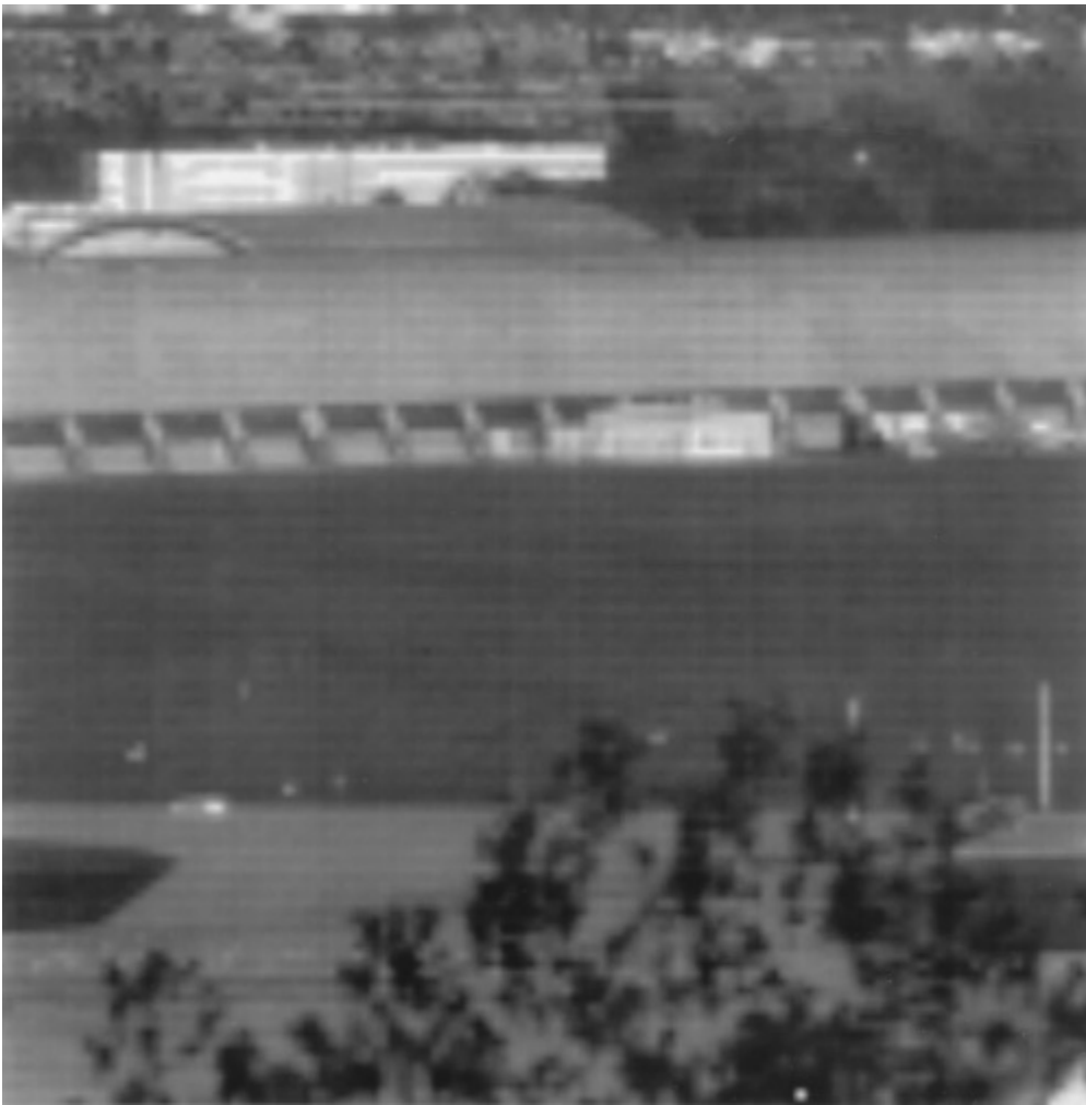
Fig. 4 Frame from Fig. 2 but with NUC by use of the initial estimates of the gain, the offset, and the noise variance.
