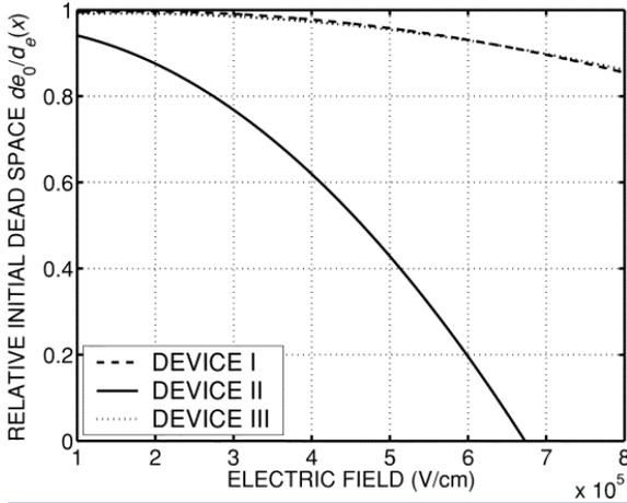
**Fig. 7.** Ratio of the injected electron's initial dead space  $d_{e0}$  to the dead space in the absence of any initial energy  $d_e(0)$  as a function of the average electric field in the multiplication region. Note that an injected carrier in Device II exhibits a significant reduction in the initial dead space from the customary (zero initial-energy) dead space, especially at high fields. In contrast, such a reduction is minimal in Devices I and III.
