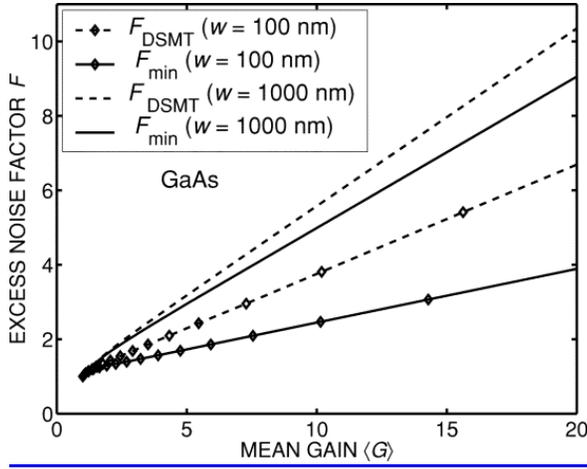
**Fig. 1.** Excess noise factor as a function of the mean gain for two GaAs APDs with multiplication-region widths of 100 nm (curves with diamonds) and 1000 nm. The solid curves represent the maximal MDSMT prediction  $F_{\min}$  for which the initial energy is set to the ionization threshold energy (i.e., zero initial dead space for the injected electron). The dashed curves are the DSMT predictions  $F_{\text{DSMT}}$ .
