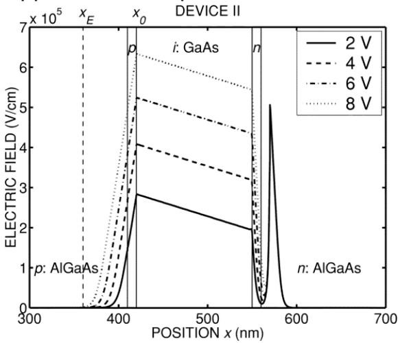
**Fig. 4.** Electric field profile for Device II. Solid vertical lines represent layer boundaries, and the dashed vertical line is used to illustrate the location  $x_E$  of the onset of the field buildup. The point  $x_0$  marks the start of the multiplication layer. The fields were calculated using MEDICI software according to the doping profiles obtained from SIMS data. Notice the extent of the spread of the field gradient to the left of the i-layer.
