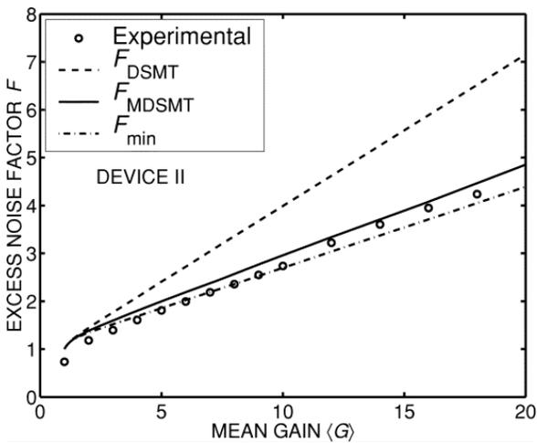
**Fig. 9.** Same as Fig. 8, but for Device II. The MDSMT model provides excellent agreement with the experimental data, while the DSMT model significantly overestimates the excess noise factor as a result of ignoring the initial energy of the injected electron.
