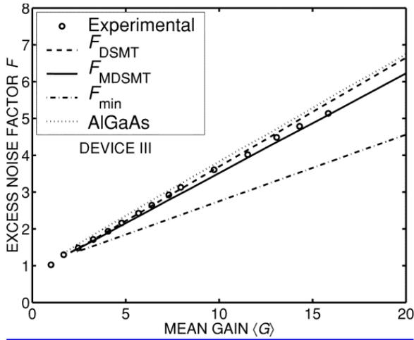
**Fig. 10.** Same as Fig. 8, but for Device III. As a result of the small initial energy, the discrepancy between the MDSMT and the DSMT predictions is small. The dotted line represents the MDSMT prediction for a hypothetical version of Device III for which both multiplication layers are  $\text{Al}_{0.6}\text{Ga}_{0.4}\text{As}$ . Ionization threshold energies for  $\text{Al}_{0.6}\text{Ga}_{0.4}\text{As}$  and the ionization-coefficients parameters were taken from [13].
