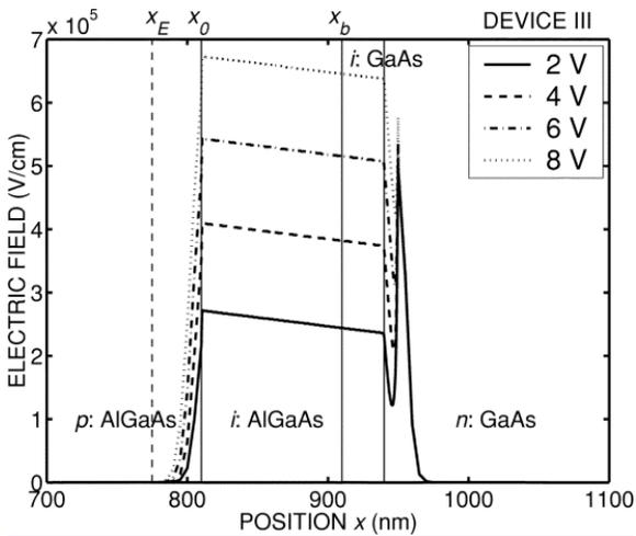
**Fig. 5.** Same as Fig. 4, but for Device III. This structure has two multiplication layers, namely,  $\text{Al}_{0.6}\text{Ga}_{0.4}\text{As}$  and GaAs.
