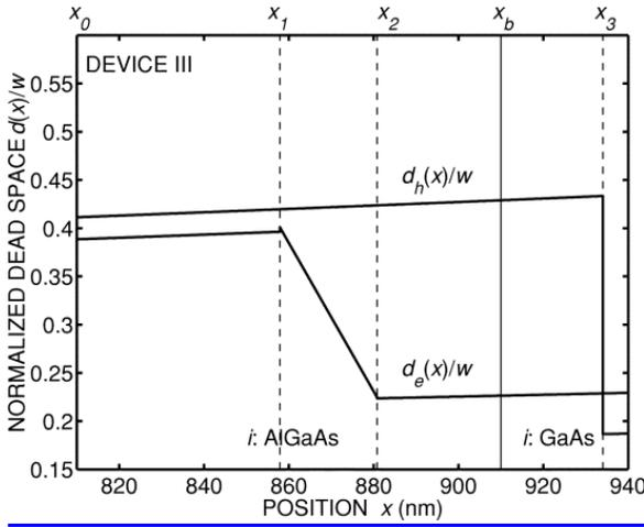
**Fig. 6.** Electron and hole dead-space profiles in the multiplication layers for Device III. The solid vertical line represents the  $\text{Al}_{0.6}\text{Ga}_{0.4}\text{As}/\text{GaAs}$  boundary.
