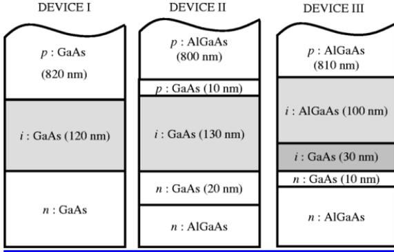
**Fig. 3.** Structure of the three APDs considered in this paper. Device I is a homostructure GaAs APD and it is used as a reference. Devices II and III are  $\text{Al}_{0.6}\text{Ga}_{0.4}\text{As}/\text{GaAs}$  heterostructure APDs, and the latter has a two-layer  $\text{Al}_{0.6}\text{Ga}_{0.4}\text{As}/\text{GaAs}$  multiplication region. Shaded areas represent the multiplication regions. Electrons are injected into the multiplication region from the top.
