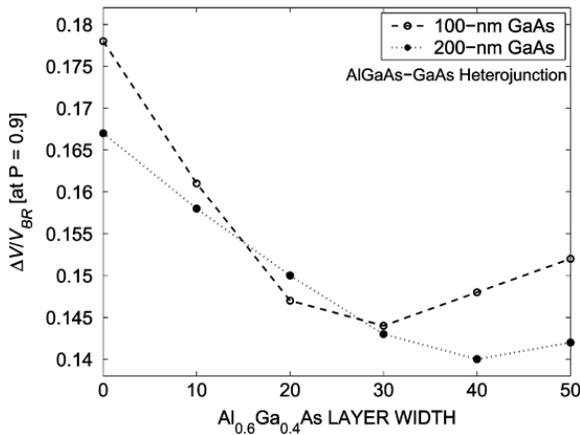
**Fig. 3.** Normalized excess voltage  $\Delta V/V_{BR}$  for achieving a breakdown probability of 0.9 as a function of the  $\text{Al}_{0.6}\text{Ga}_{0.4}\text{As}$  layer width. The dashed curve with open circles ( $\circ$ ) represents the 100-nm GaAs APD and the dotted curve with closed circles ( $\bullet$ ) represents the 200-nm GaAs APD.
