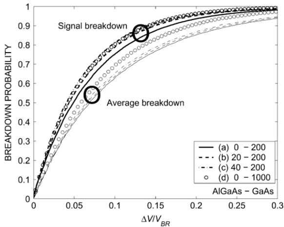
**Fig. 2.** Breakdown probability of 200-nm GaAs with (a) no  $\text{Al}_{0.6}\text{Ga}_{0.4}\text{As}$  layer (solid), (b) a 20-nm  $\text{Al}_{0.6}\text{Ga}_{0.4}\text{As}$  layer (dashed), (c) a 40-nm  $\text{Al}_{0.6}\text{Ga}_{0.4}\text{As}$  layer (dashed-dotted), (d) a 1000-nm homojunction GaAs (○). Thin curves represent the average breakdown probability caused by randomly-distributed dark carriers.
