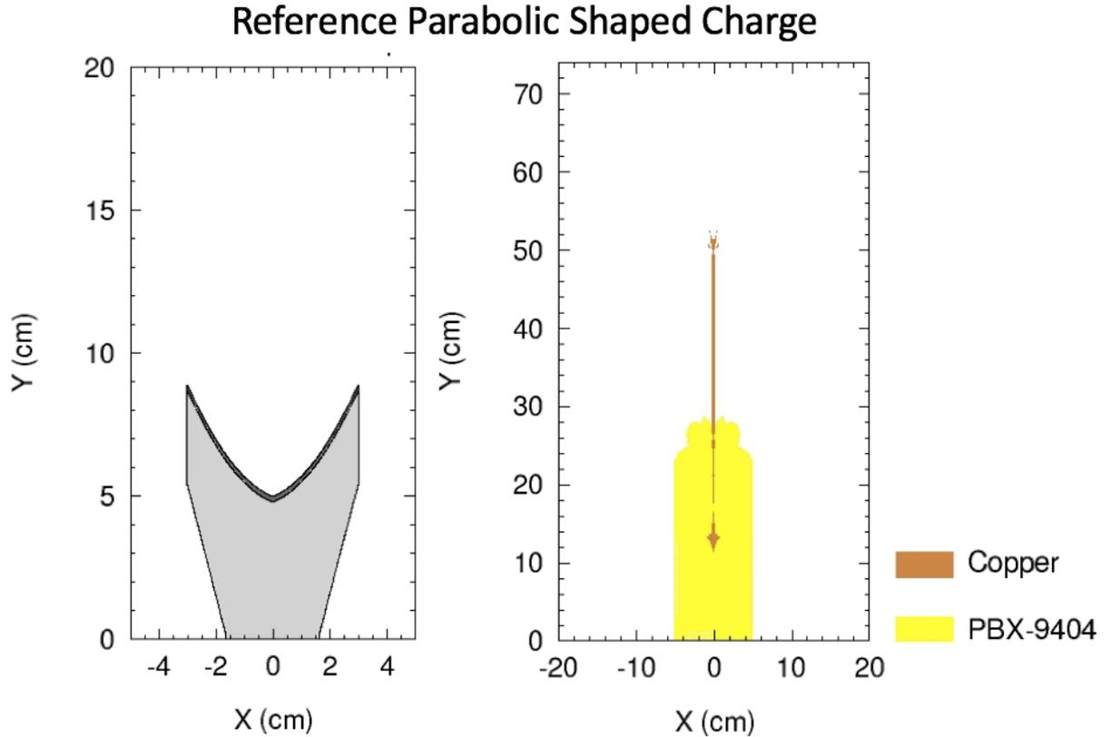
Figure 7: An illustration of the reference shaped charge geometry corresponding jet. Thickness is 0.20 cm  $a=0.30$   $b=0.40$   $c=5.00$
