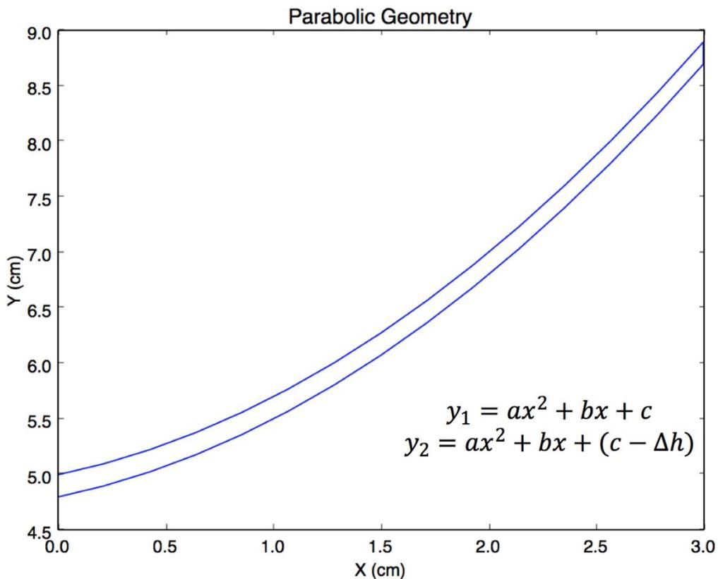
Figure 3-A: A plot of the parabolic shaped charge liner
