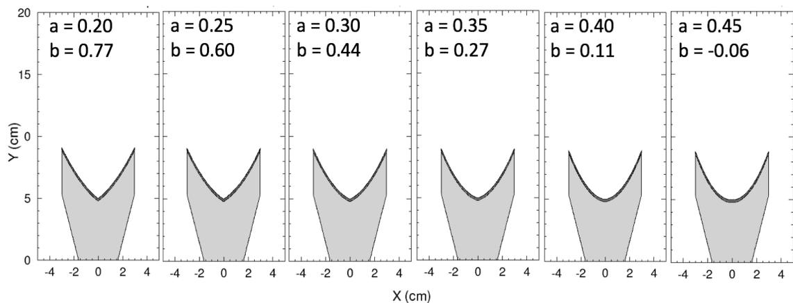
Figure 18: Displayed above are different shaped charge geometries with their respective  $a$  and  $b$  values generated from  $b = -3.291 a + 1.424$ .
