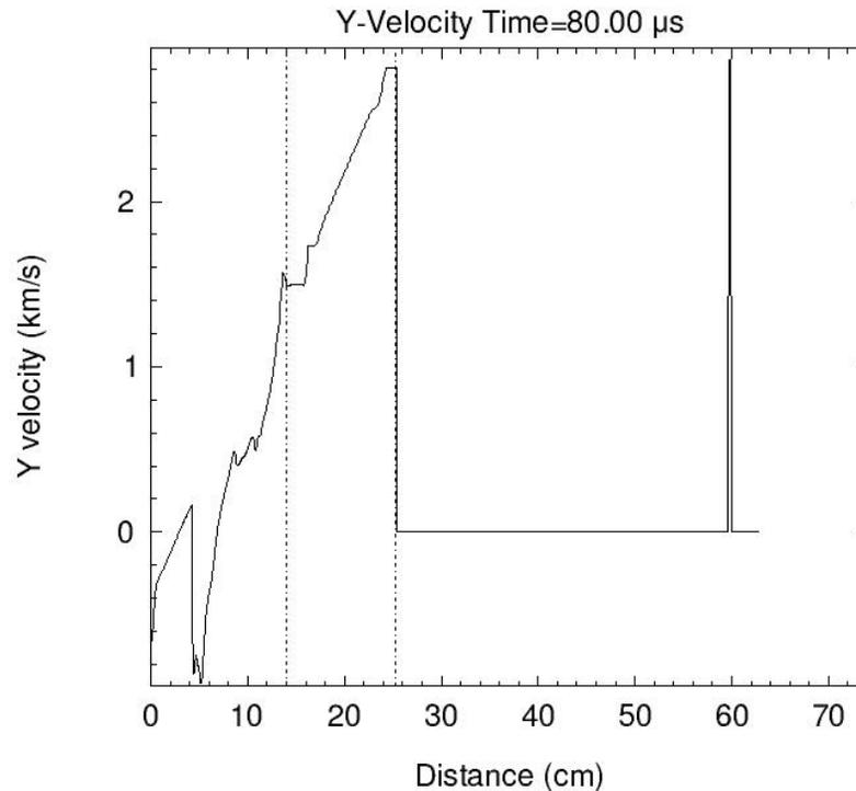
Figure 11: A plot showing the y - velocity profile (from a tracer) of the problematic SC jet. Observe that it does not meet the three km/s minima to write to the data dump file.
