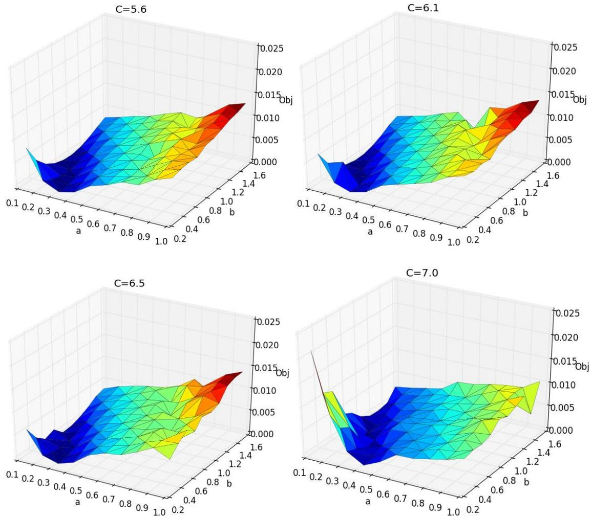
Figure 13: A collection of surfaces varying  $c$  showing relationships between  $a$ ,  $b$  and  $OF$ . Recall that one seeks to minimize the  $OF$  therefore dark blue areas are target points. The first plot's axis has been changed to match the rest of the plots. Original plots are shown in the appendix.
