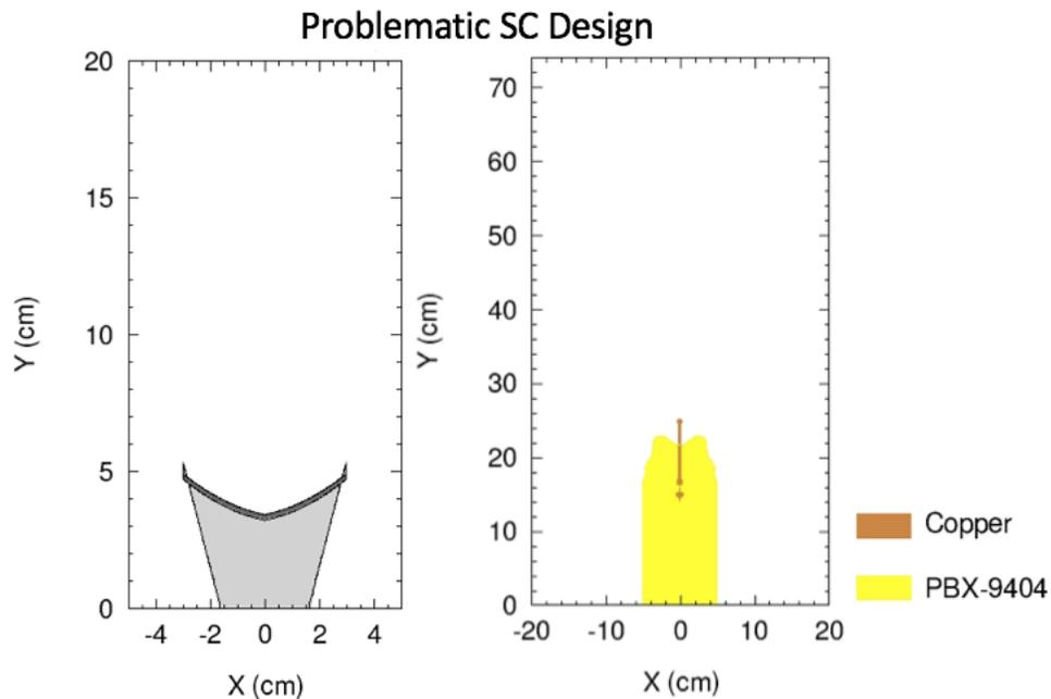
Figure 10: An illustration of poor liner geometry and corresponding jet. Observe the underdeveloped shaped charge jet. The parameters used for this simulation were  $a = 0.10$ ,  $b = 0.20$ ,  $c = 3.00$ .
