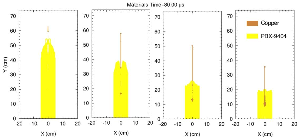
Figure 8: Illustrations of the shaped charge jet procured from various thicknesses. From left to right, thicknesses of 0.05, 0.10, 0.20, 0.50 cm
