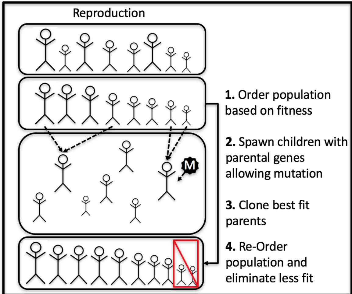
Figure 3: A schematic of the reproduction cycle in a genetic algorithm. Adapted from the Dakota Reference Guide.
