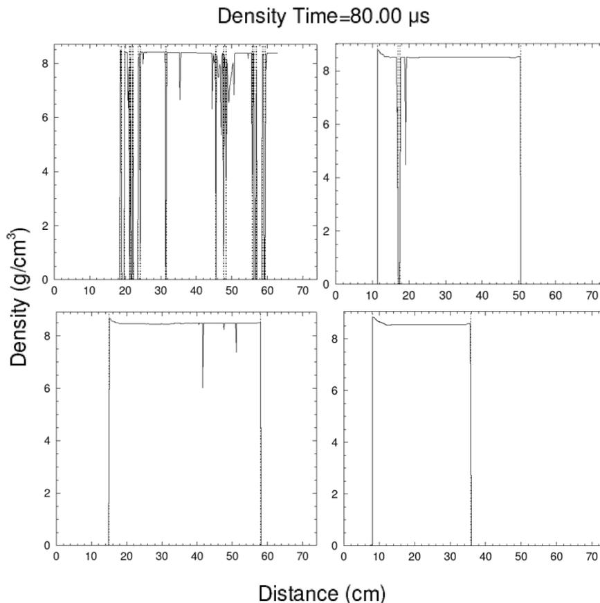
Figure 9: A comparison of density versus distance of shaped charge jets of varying thickness. Upper left,  $t=0.05$  cm, upper right  $t=0.20$  cm, lower left  $t=0.10$  cm, lower right  $t=0.50$  cm
