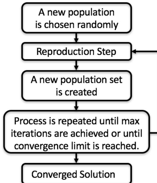
Figure 2: A schematic of a genetic algorithm
