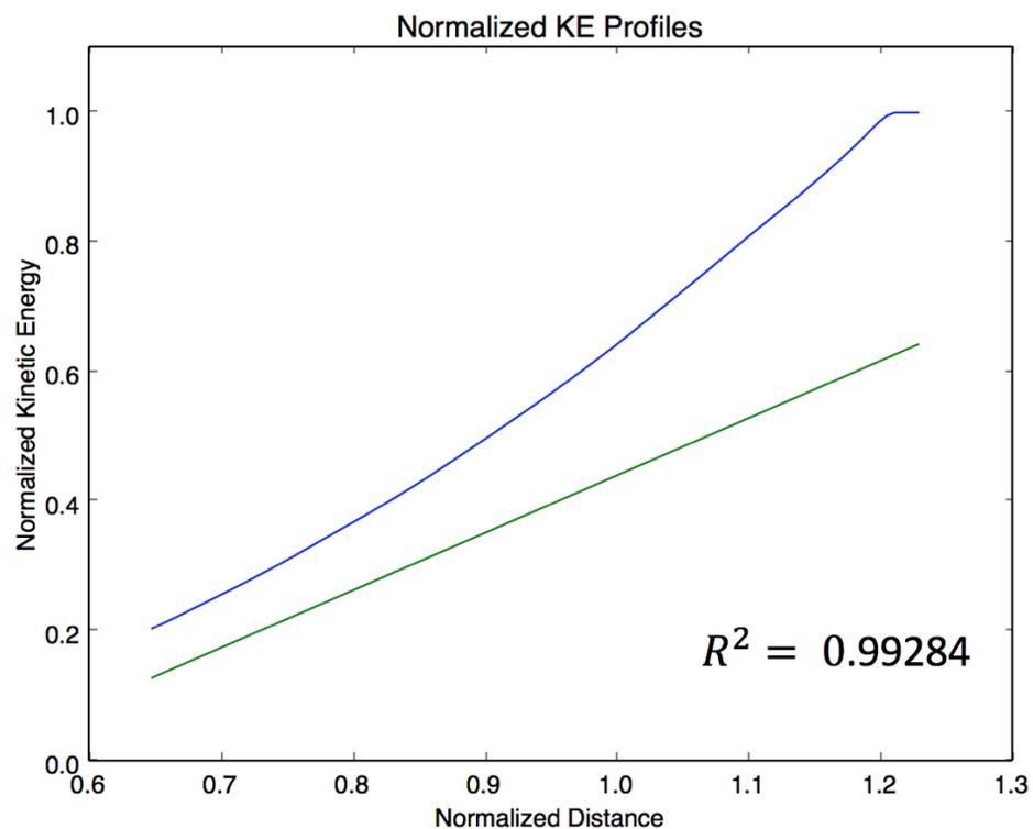
Figure 6: An illustration of the linear regression between two normalized kinetic energy profiles. The blue is the normalized KE profile and the green is the reference KE profile generated by the target shaped charge geometry.
