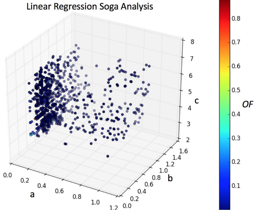
Figure 21: A scatterplot illustrating the trial points chosen by the Soga algorithm. The color scale displays the value of the linear regression objective function
