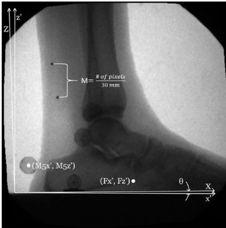
**Figure 3.** Fluoroscopic image showing a point of interest location that is translated from image coordinates ( $Fx'$ ,  $Fz'$ ) to global coordinates using an external marker image ( $M5x'$ ,  $M5z'$ ) and global coordinate locations, as well as the image magnification factor ( $M$ ), subject foot progression angle (calculated from external marker  $M5$  and  $M6$  global coordinates), and camera static angular rotation from global ( $\theta$ ).
