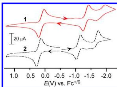
**Figure 3.** Cyclic voltammograms of **1** and **2** in  $\text{CH}_2\text{Cl}_2$  with  $0.1 \text{ M}$   $(\text{NBu}_4)\text{PF}_6$  as the supporting electrolyte.
