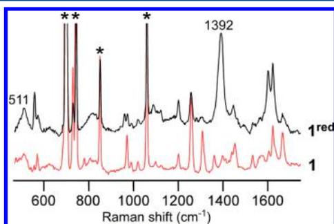
**Figure 5.** rR spectra obtained with 413.1 nm excitation (40 mW) of  $1^{\text{red}}$  (black) and **1** (red) in frozen  $\text{CD}_2\text{Cl}_2$  solutions. Peaks with an asterisk (\*) arise from solvent.
