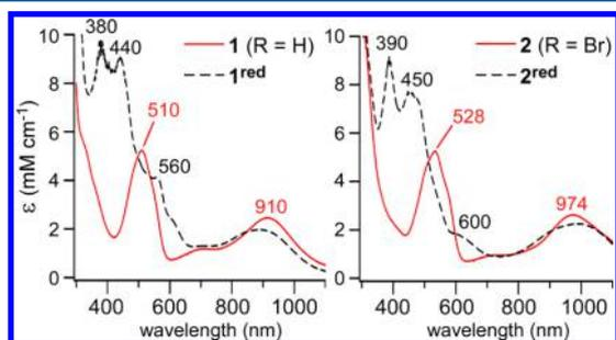
**Figure 2.** Red, solid lines: UV–vis absorption spectra of **1** and **2** in  $\text{CH}_2\text{Cl}_2$  at room temperature. Black, dashed lines: Spectra measured after the addition of 1 equiv of  $\text{CoCp}^*_2$  (**1**) or  $\text{CoCp}_2$  (**2**) at  $-30$  °C in  $\text{CH}_2\text{Cl}_2$  to give the corresponding  $X^{\text{red}}$  species.
