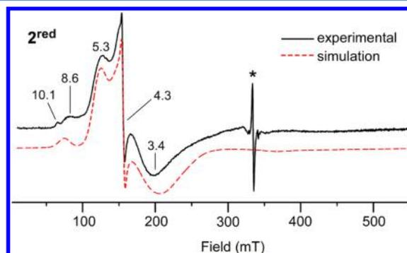
**Figure 4.** X-band EPR spectrum of  $2^{\text{red}}$  in frozen  $\text{CH}_2\text{Cl}_2$  at  $20 \text{ K}$ . The sharp feature (\*) arises from a radical impurity. Simulation of the data required two  $S = 5/2$  species with the following parameters: major (92%),  $D = -4.0 \text{ cm}^{-1}$ ,  $E/D = 0.18$ ,  $g = 2.0, 2.0, \text{ and } 2.1$ ; minor (8%),  $D = 1.6 \text{ cm}^{-1}$ ,  $E/D = 0.33$ ,  $g_{\text{iso}} = 2.0$ .
