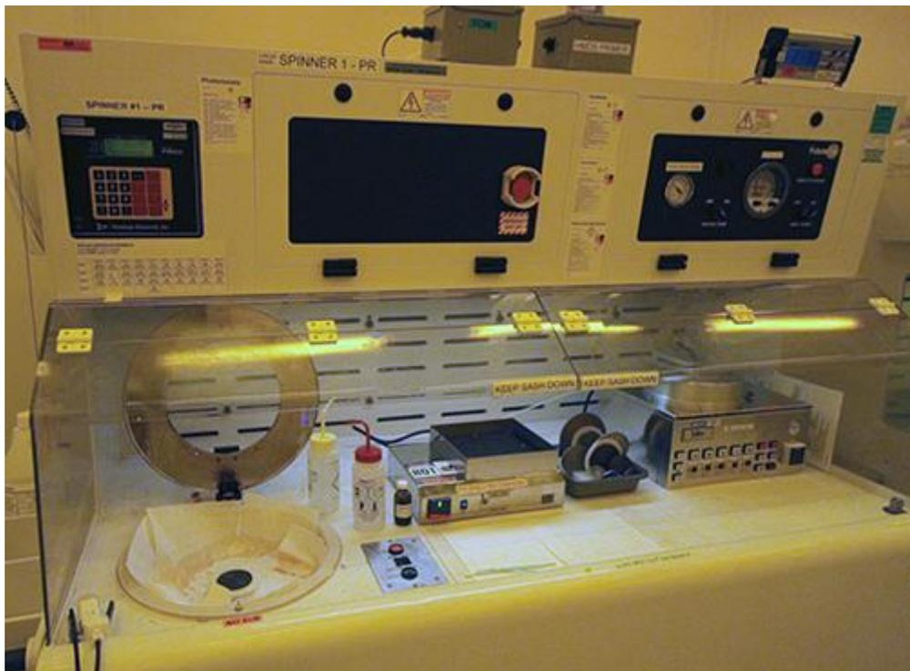
**Figure C-2.** Solvent hood at the University of Wisconsin-Madison, The Nanoscale Fabrication Center (NFC) used for photolithography and cleaning.
