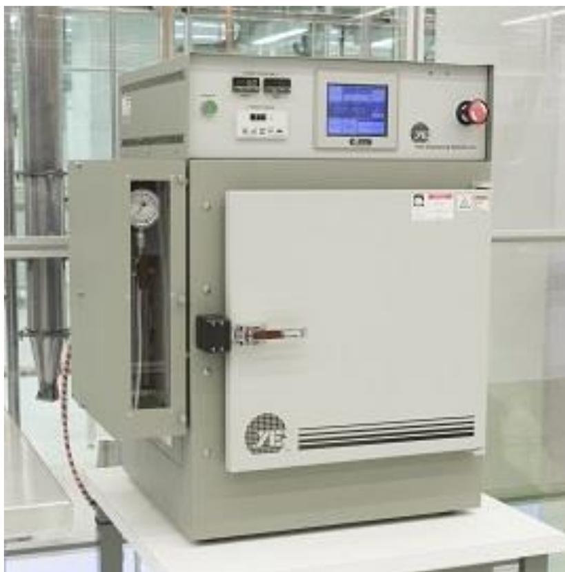
**Figure C-1.** YES-58TA Vacuum Bake/HMDS Vapor Prime and Image Reversal System.
