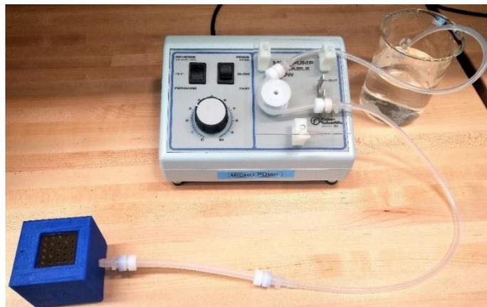
**Figure 77.** Setup for water flow testing.
