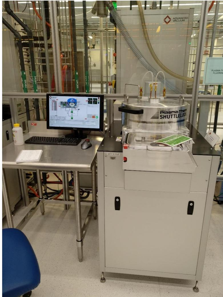
**Figure C-9.** Plasma-Therm ICP Fluoride Etch at University of Chicago, The Pritzker Nanofabrication Facility. We etched out silicon nitride and silicon oxide layer to get our desired pattern.
