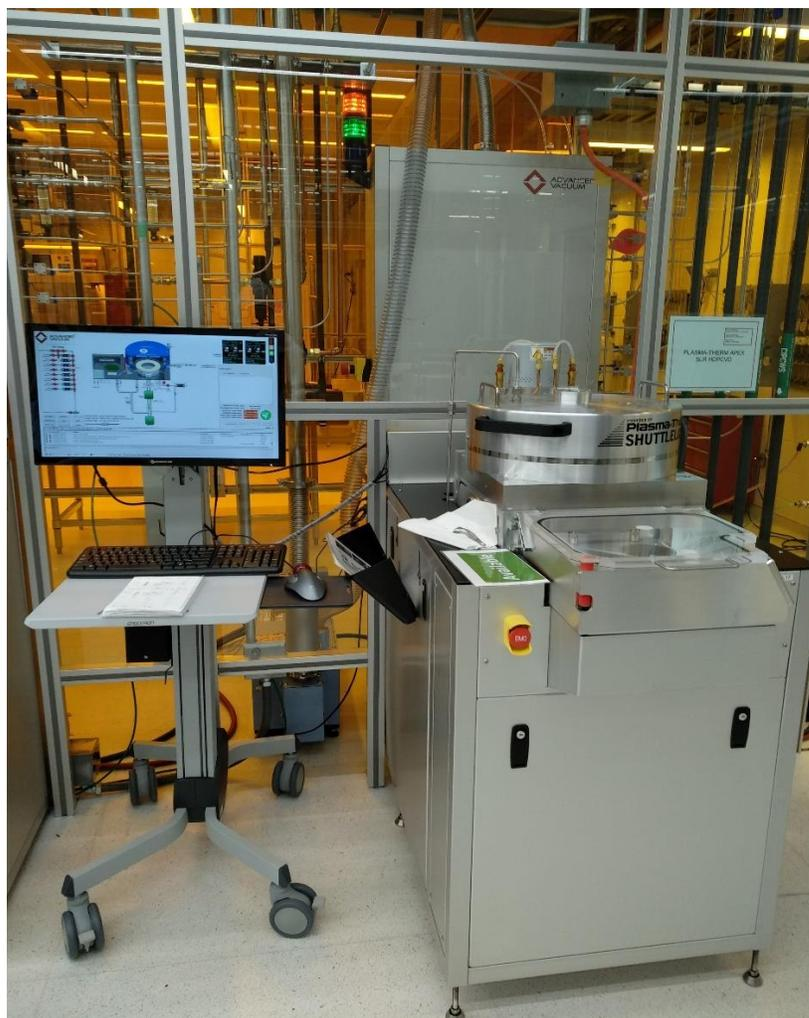
**Figure C-8.** Plasma-Therm Apex SLR HDPCVD.
