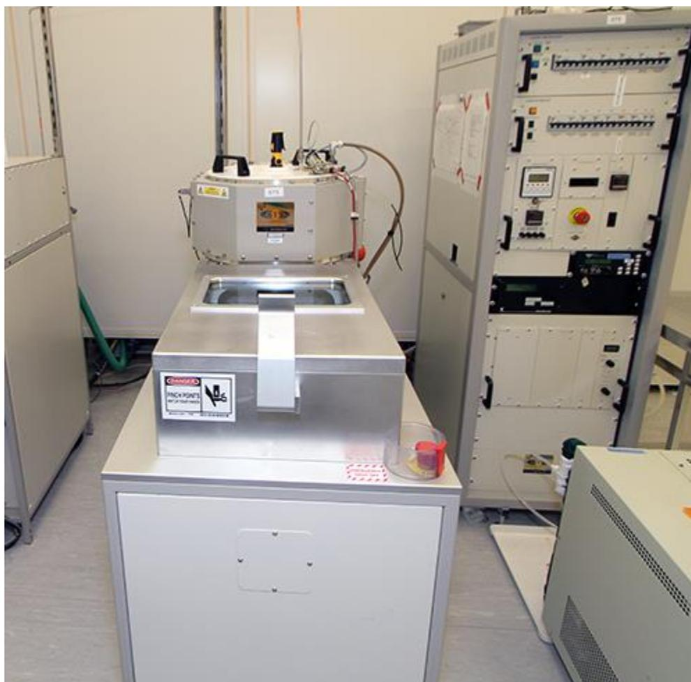
**Figure C-5.** STS Deep Reactive Ion Si Etcher at the University of Wisconsin-Madison, The Nanoscale Fabrication Center (NFC). For our recipe, the Si etch rate was  $\sim 2.31$   $\mu\text{m}/\text{min}$ .
