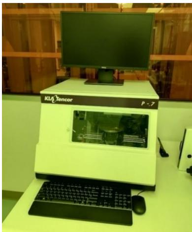
**Figure C-12.** KLA-Tencor P-7 Surface Profilometer.
