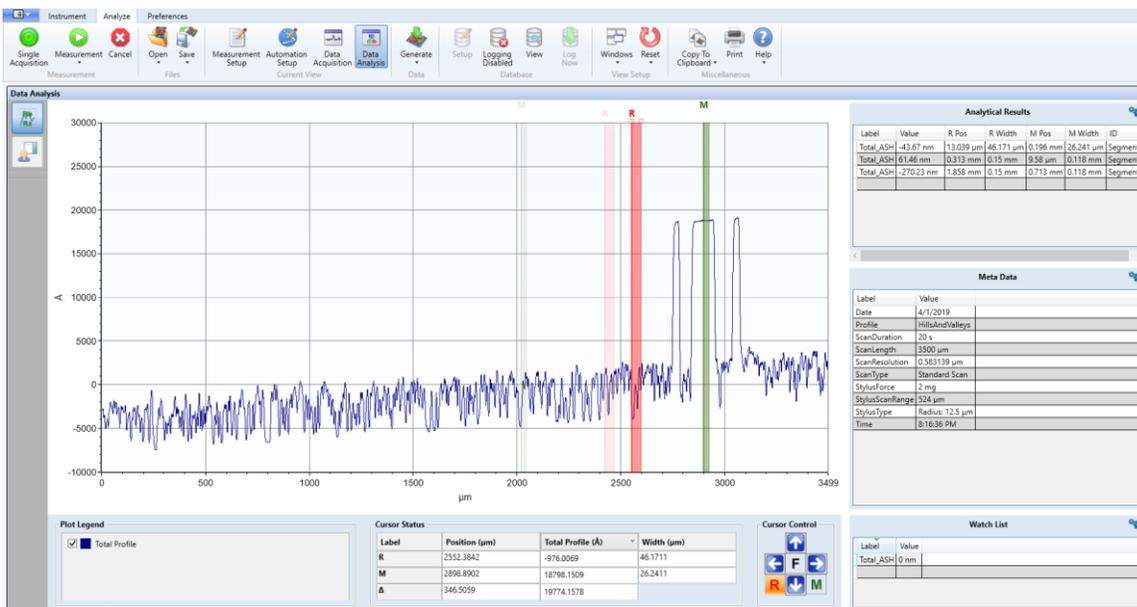
**Figure 30.** SiO<sub>2</sub> and Si<sub>3</sub>N<sub>4</sub> thickness measurement using Bruker Dimension Icon AFM profilometer.
