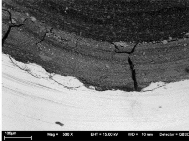
Fig. 9. ESEM of zirconia crown showing 3 core chips. In this view, die material is at *top*, cement in *middle*, and zirconia core at *bottom*. Original magnification  $\times 500$ .
