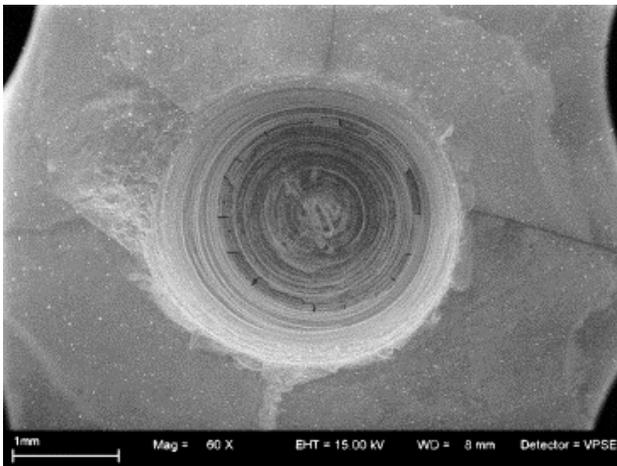
Fig. 7. ESEM of zirconia crown showing radial crack formation from access. Variable pressure [secondary electron](#) (VPSE, bottom right) detector was used in obtaining this image. Original magnification  $\times 60$ .
