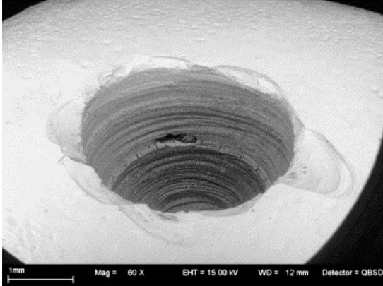
Fig. 4. ESEM of alumina crown showing significant chip as well as edge chipping within veneering [porcelain](#). Backscattered electron (QBSD, bottom right) detector was used in obtaining this image. Original magnification  $\times 60$ .
