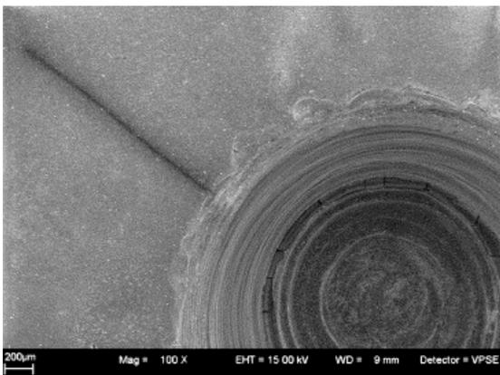
Fig. 8. ESEM of zirconia crown showing close-up view of radial crack formation from access. Original magnification  $\times 100$ .
