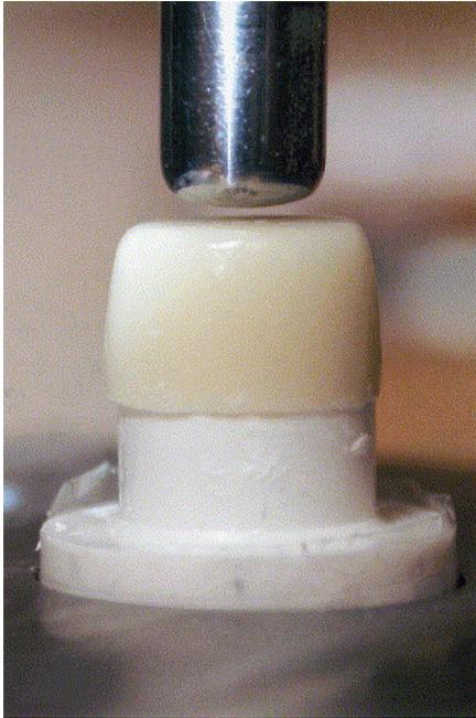
Fig. 3. Loading piston was 6.35 mm in diameter along its long axis, with its end machined to curvature equivalent to 50 mm in diameter, which contacted center and approximate same area of each crown.
