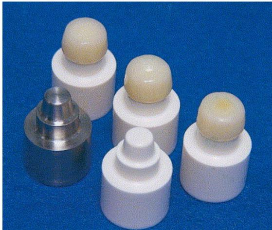
Fig. 2. Stainless steel master die and duplicated high-heat epoxy die (left to right, front diagonal row). Intact alumina crown, accessed alumina crown, and repaired alumina crown (left to right, back diagonal row).
