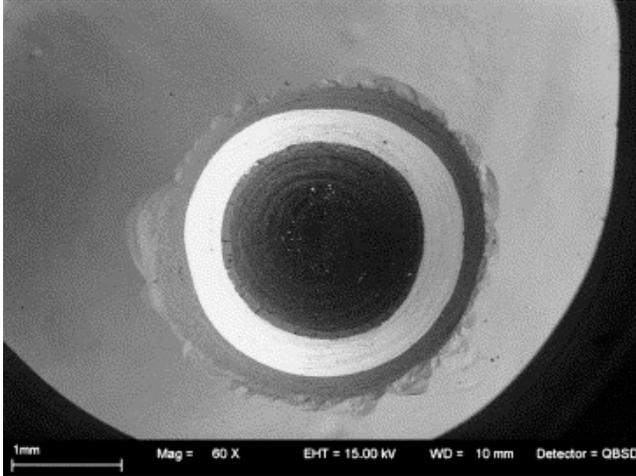
Fig. 6. ESEM of zirconia crown showing edge chipping. Zirconia core is area in *white*. Original magnification  $\times 60$ .
