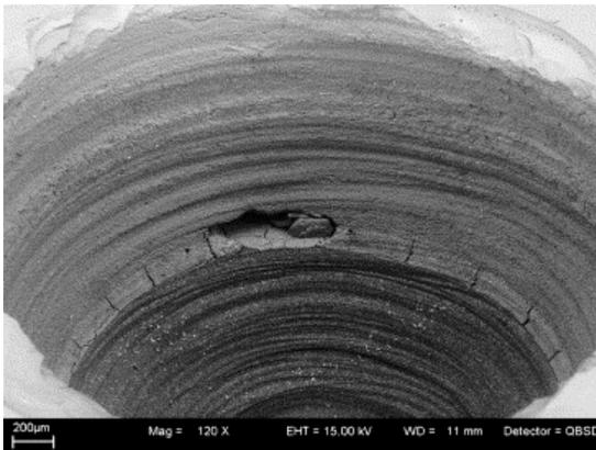
Fig. 5. ESEM of alumina crown showing void in cement layer that appears to extend into core, indicating that section of core chipped away during [endodontic](#) access procedure. Original magnification  $\times 120$ .
