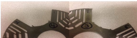
Figure 16: Close-up images of the failed laminates, indicating the point of failure at the bridges and posts.
