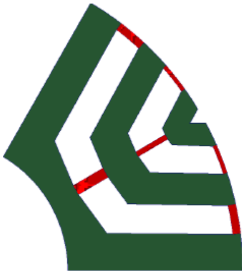
Figure 1: Cross-section of synchronous reluctance design using dual phase material, red-non-magnetic, green-magnetic
