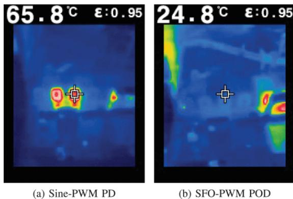
Fig. 8. Infrared Images of the NPB switches  $S_{r2}$  and  $S_{r3}$  at 15kW load under various modulation methods
