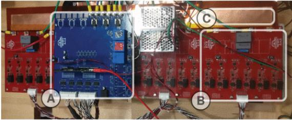
Fig. 5. Experimental prototype of the customized A3L-ANPC converter, (A) control board, (B) Phase-A leg, (C) the dc-bus bar
