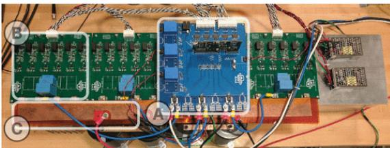
Fig. 6. Experimental prototype of the A3L-ATT converter, (A) control board, (B) Phase-A leg, (C) the dc-bus bar
