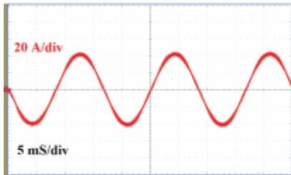
(b) Load current (Phase-A) with Sine-PWM PD (20A/div)
