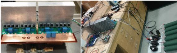
Fig. 4. Experimental prototype of the fault tolerant t-type converter
