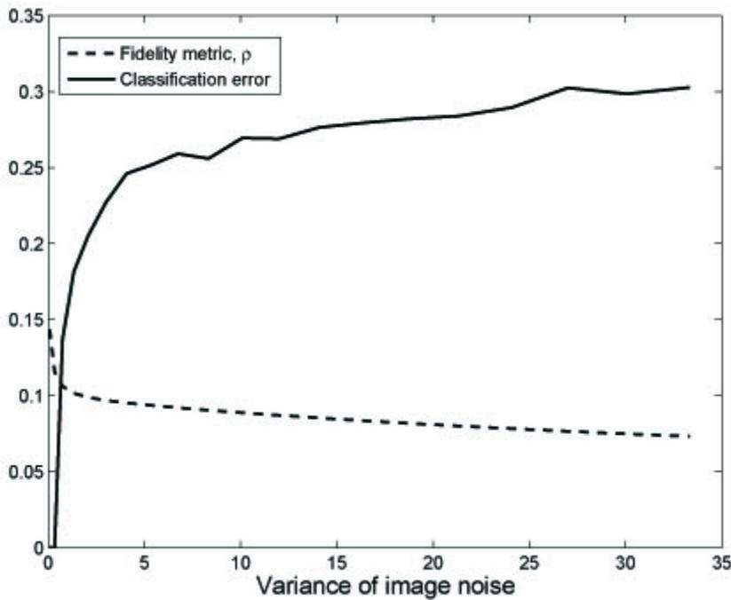
**Fig. 4.** Figure showing the fidelity metric,  $\rho$ , and the classification error versus the noise variance in the input image. The classifier is run for 10,000 times for each value of noise variance to average out the classification error. Here  $N_p \epsilon = 0.3$ .
