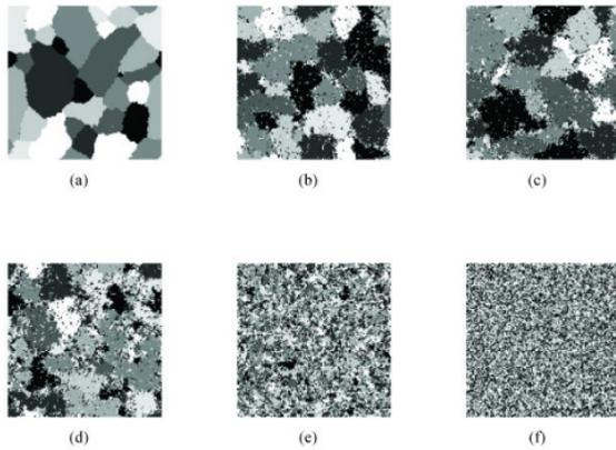
**Fig. 9.** Sample MRF images generated according to a generalized Ising model with potential energies given by (18) using various values for the parameter  $\beta$ . We employed a Metropolis sampler using 1000 iterations. The values used for the parameter  $\beta$  are (a)  $\beta = -2$ , (b)  $\beta = -1$ , (c)  $\beta = -0.975$ , (d)  $\beta = -0.95$ , and (e)  $\beta = -0.9$ , (f)  $\beta = -0.4$ .
