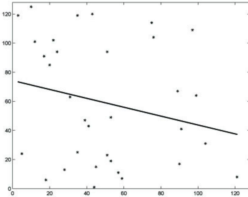
**Fig. 3.** Figure showing the output 128x128 photon-counted array, where the photon counts are represented by the symbols ‘\*’, and the best-fit estimate of the line from the photon counts. The value of  $k$  is 5 and the corresponding noise variance is 2.08. Here  $N_p \epsilon = 0.3$ .
