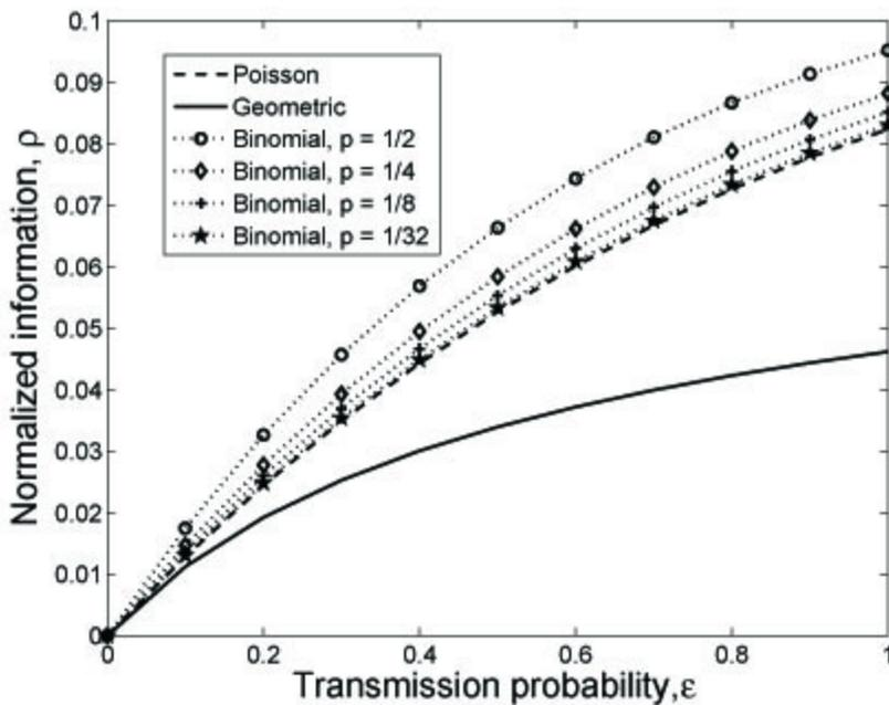
**Fig. 6.** Normalized mutual information for different possible channel distributions while using a Markov-chain model for  $P_{\mathbf{x}(\mathbf{x})}$ , with a specific correlation index,  $m = 0.01$ . Here we used  $N_p = 3$ .
