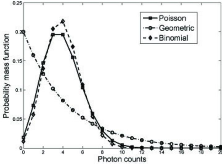
**Fig. 2.** This figure shows Poisson, geometric and binomial probability mass functions. The various parameters used are  $\lambda = 4$  for Poisson,  $p = 0.2$  for geometric, and  $n = 20, p = 0.2$  for binomial. In all three cases the mean value is 4.
